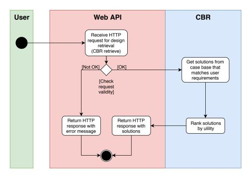
Figure 4.7: Activity diagram that shows the activity flow of the retrieval process
