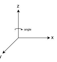
**Figure 4.6:** The coordinate system used in Winner Design is left-handed where the z-axis points up and the x-axis points to the right. Rotation in a left-handed coordinate system is clock-wise.
