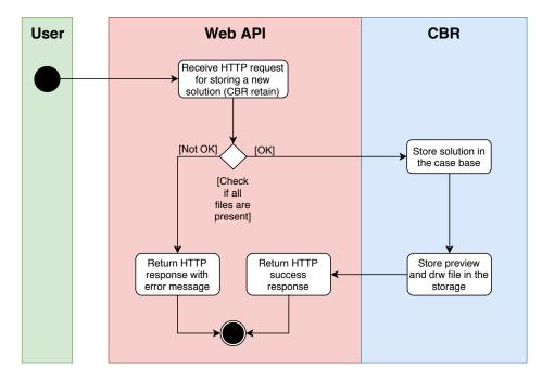
Figure 4.8: Activity diagram that shows the activity flow of the retain process
