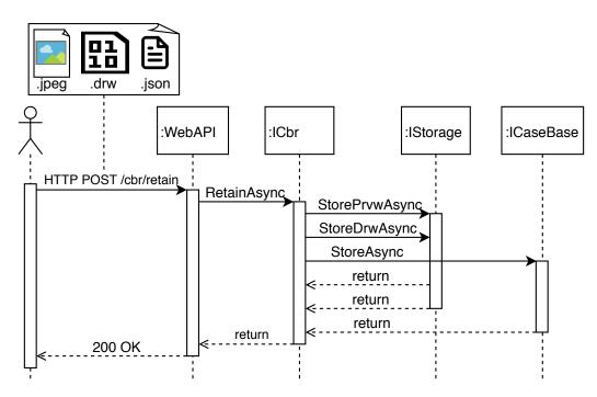
**Figure 4.10:** Sequence diagram that shows the program flow when using the /cbr/retain endpoint.
