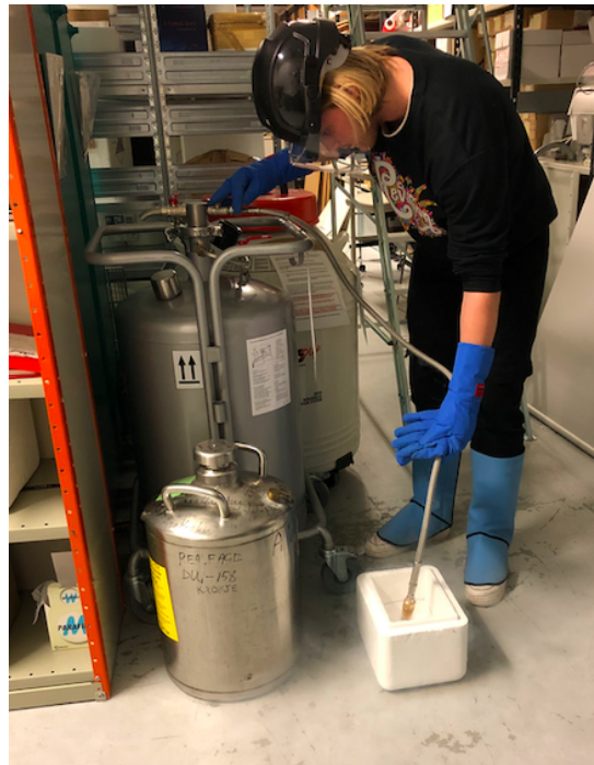
Figure A.1.2: Poring liquid nitrogen
