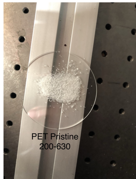
(d) PET Pristine, smaller than 630, but larger than 200 micron
