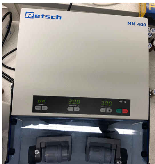
Figure A.1.3: Pulverizing plastic in the tissue lyser
