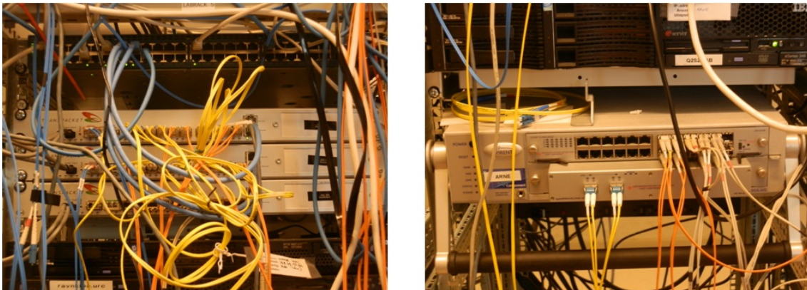
Figure 8.1: Left: Optical connections made in H1 nodes; mainly loops and the 10GE connection between each other. Right: Spirent node and its optical connections to the H1 nodes.
