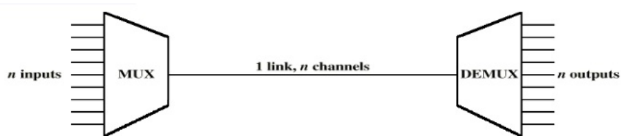
Figure 2.2: A MUX-DEMUX example.
