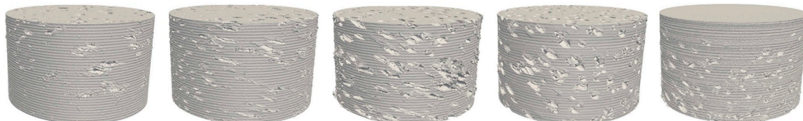
Fig. 3. 3D rendering of the XRMCT data sets of one of the porous specimen series (specimens with origin e to a are printed from left to right, respectively).
