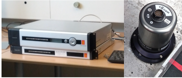
Figure 4.2: The Seapath 330+ navigation system, which consists of a processing unit, an interface unit and an IMU, in addition to cabling and GNSS antennas not shown in the photo.
