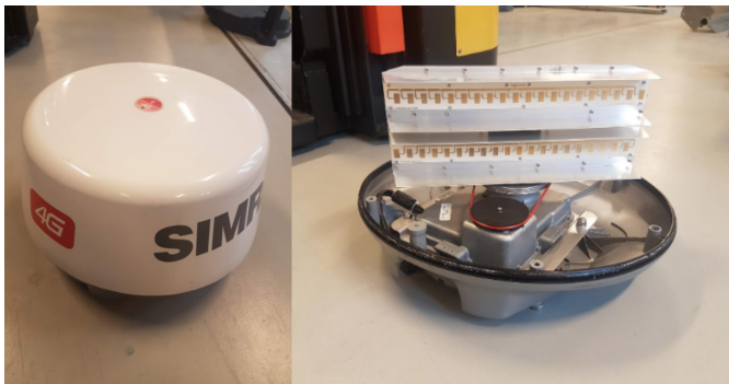
Figure 4.1: The Navico Simrad 4G radar, with and without the dome.
