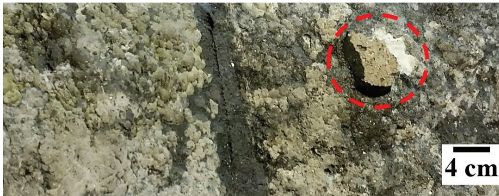
Figure 4.32. Pitting on the cathode surface surrounding the pothole that led to tapout of pot 3. Red dashed circle highlights the tapout hole.
