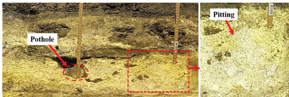
Figure 4.56. Pitting on the cathode surface of pot 6. The pothole and pitting locations are highlighted in the figure.
