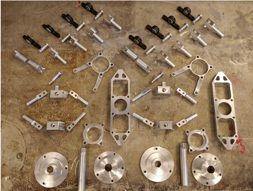
Figure 4.11: An overview of the main parts of the suspension system.
