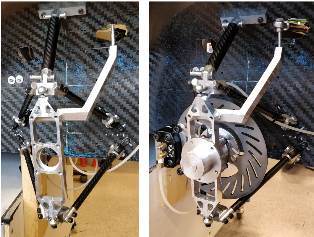
(a) Demonstration of the mounted suspension arms and steering knuckle front layer.
