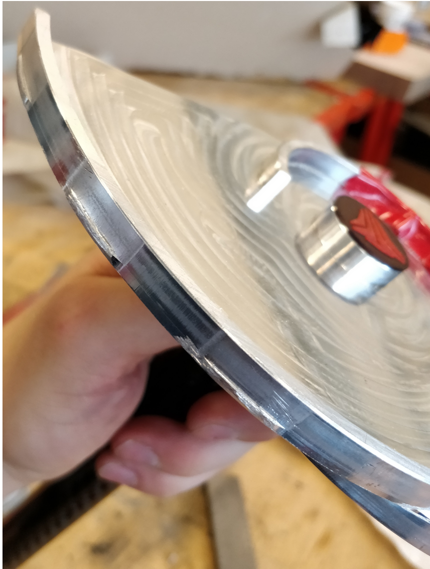
Figure 3.15: The indentations caused by the machining of the tabs. The edge in the lower right corner of the photo is where the roller pins caught on.
