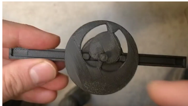
Figure 3.4: Implementation prototype of double-guide wheel concept. (click the figure or caption to see a motion animation)
