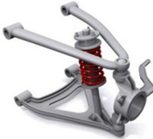
Figure 2.9: Example of a double wishbone suspension system. [24]
