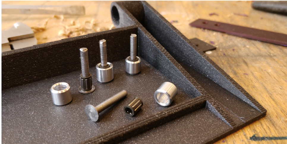
Figure 3.13: The rollers, pins and bearings.
