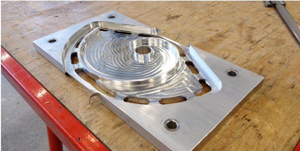
Figure 3.12: The double-guide wheel straight out of the CNC milling centre.
