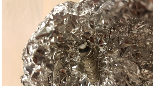
Figure 4.4: Burnt out crucible. The tungsten wire has clearly burnt itself into the ceramics, this is suspected to be the source of oxygen when evaporating.
