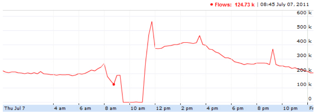
Figure 2.1: Illustration of the effect a DDoS attack can have on network infrastructure
