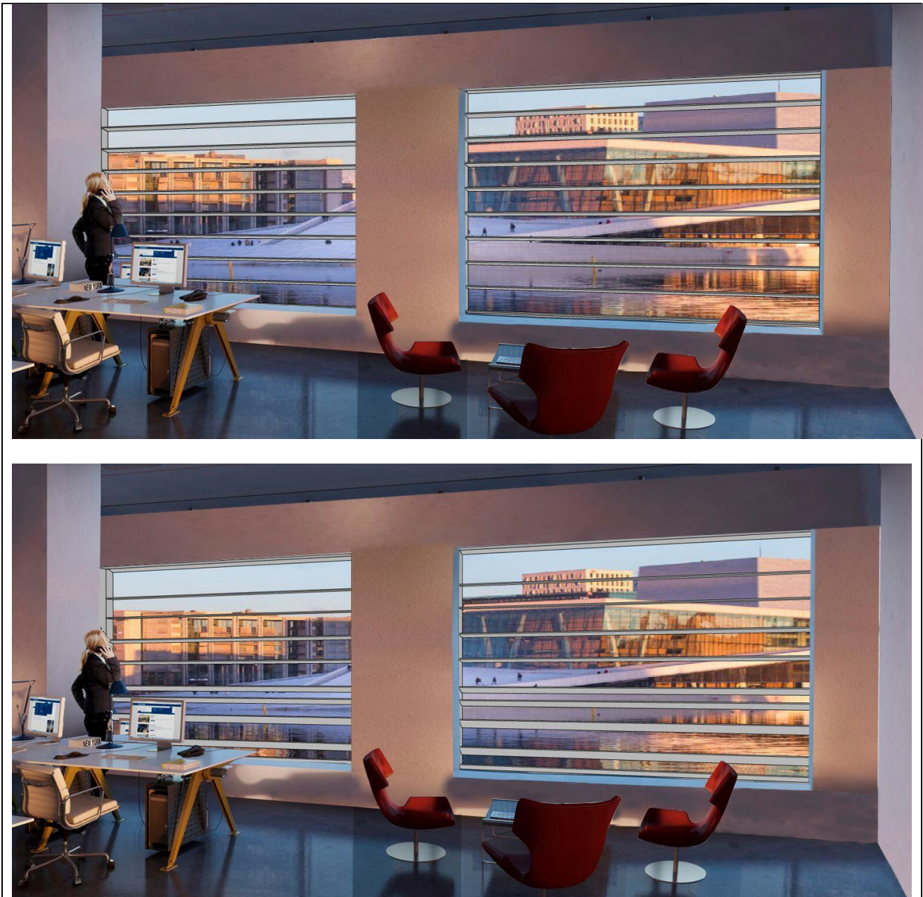
Figure 17 Side-by-side rendering of the reference case (top) with 10 louvres and the Pareto optimized configuration (bottom).
