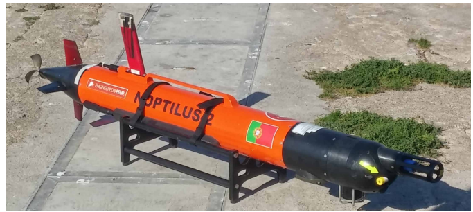
Fig. 10: Light autonomous underwater vehicle (LAUV).
