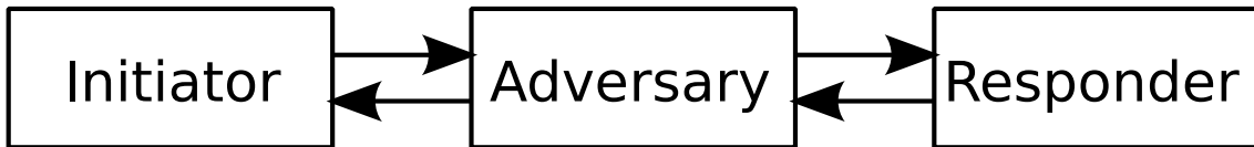
Figure 4.1: Protocol model with initiator and responder. The adversary is modeled as the network. The adversary can read, replay or forge every unprotected protocol message. The adversary cannot delete or intercept (i.e. read and delete) protocol messages.
