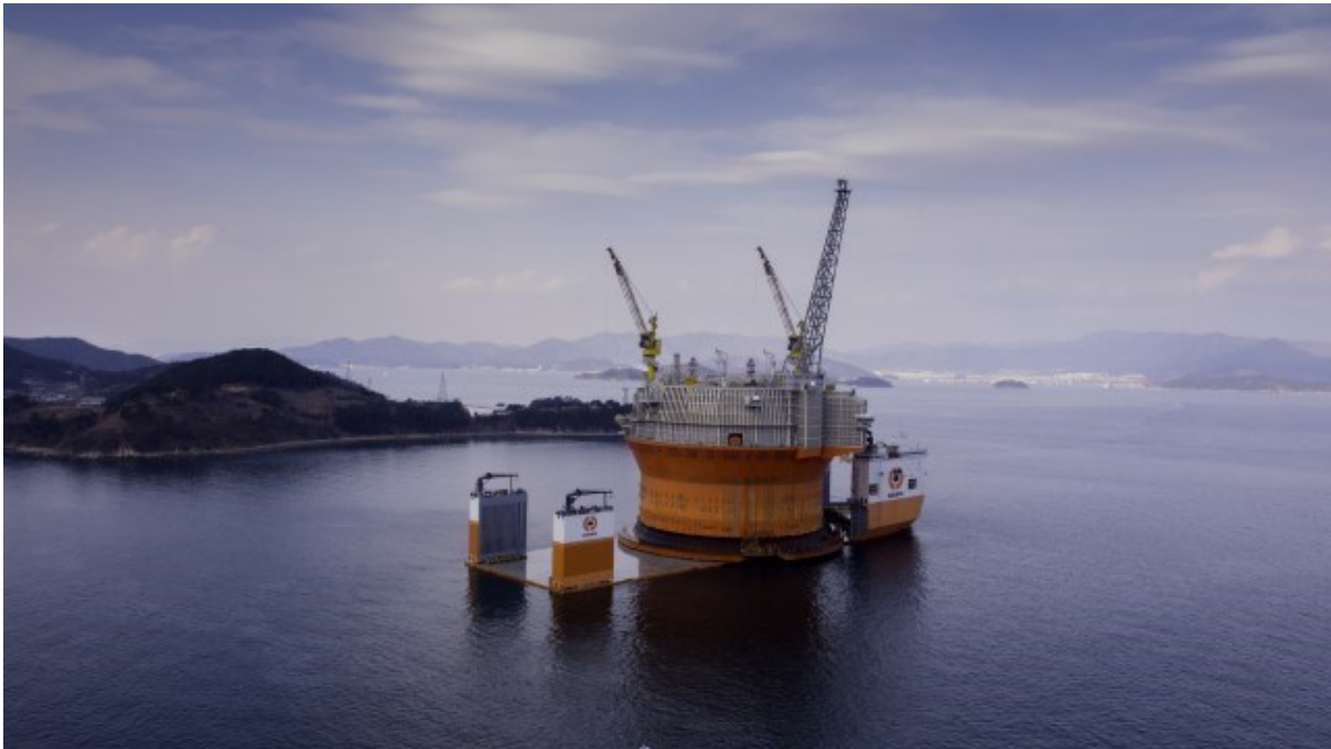
Figure 3.2 Sevan 1000 FPSO during the transportation operation (Sevan SSP, 2019)
