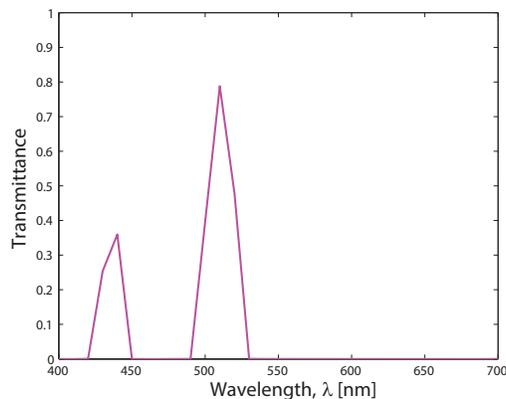
Fig. 2. Spectral transmittance of the Omega XF1078 filter.
