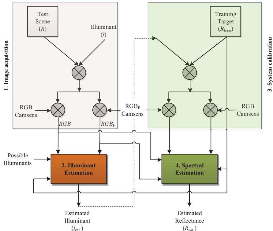
Fig. 1. Framework for the spectrogenic imaging system.
