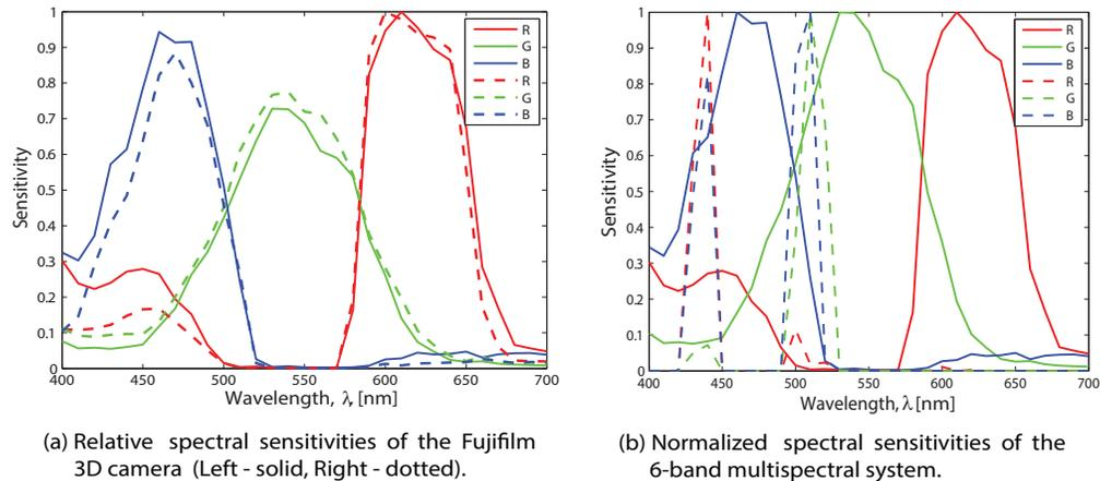
Fig. 3. Spectral sensitivities of the individual cameras, and the 6-channel multispectral system.
