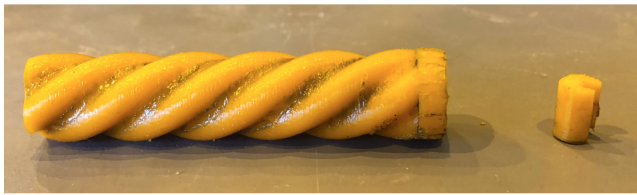
Figure 7.23: Rotor coupling failure.
