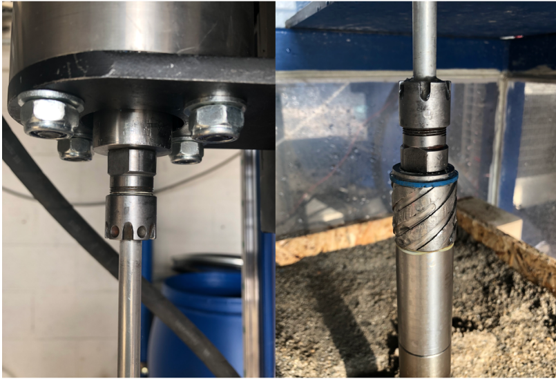
Figure 7.54: (Left) Top drill pipe connection. (Right) Bottom drill pipe connection.
