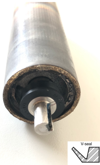
Figure 7.33: V-seal on the electric motor shaft. When pressurized this seal makes contact with the plate where the motor sits and prevents any water from going further inside the housing.
