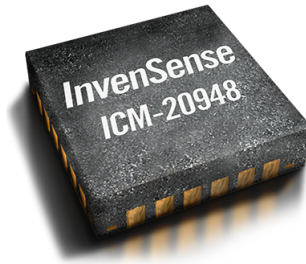
Figure 9.22: TDK InvenSense ICM-20948 9-axis IMU [18]
