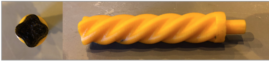
Figure 7.20: New rotor 3D-printed in PLA. Notice the four lobes following a spiral along the rotor. This feature provides more torque and less rpm to the power section.
