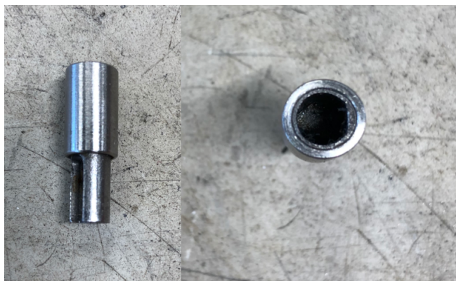
Figure 7.28: Different views of the reinforced coupling. On the right, the coupling has taken a slight oval shape enough to cause issues with the rest of the transmission.
