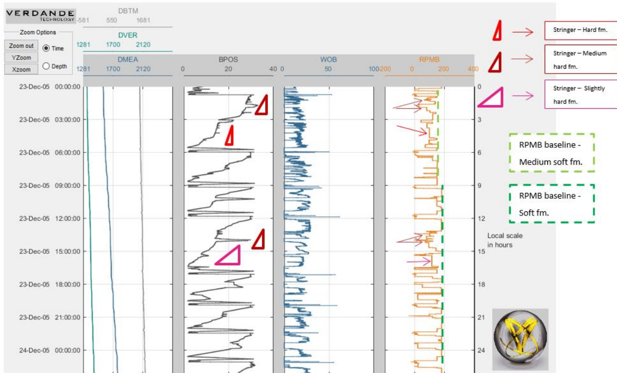
Figure 5.3: RTDD from Well C-47 bit section 17 ½" dated 23 December 2005. DBTM, DVER and DMEA are drilling depth data measured vs. time. BPOS, WOB and RPM are also plotted vs. time in different real-time drilling windows. Green stapled lines indicate RPMB baselines for a soft (dark green) and medium soft (light green) formation. Red right triangles (showing BPOS speed by their inclination/steepness) and red arrows (showing corresponding RPMB) indicate where hard stringers are located. Bright red marks a stringer for a hard formation (section 1 only), dark red marks stringers for a medium hard formation (section 1 and 4) while pink marks stringers for a slightly hard formation (section 4 only).
