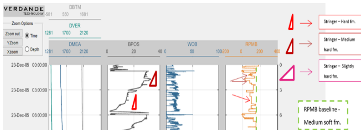
Figure 5.16: RTDD from Section 1, 1567-1594 m MD. DBTM, DVER and DMEA are drilling depth data measured vs. time. BPOS, WOB and RPM are also plotted vs. time in different real-time drilling windows. Green stapled lines indicate RPMB baselines for a soft (dark green, not shown here) and medium soft (light green) formation. Red right triangles (showing BPOS speed by their inclination/steepness) and red arrows (showing corresponding RPMB) indicate where hard stringers are located. Bright red marks a stringer for a hard formation (section 1 only), dark red marks stringers for a medium hard formation (section 1 and 4) while pink marks stringers for a slightly hard formation (section 4 only, not shown here). Hard stringers are indicated at least at three locations in Section 1.
