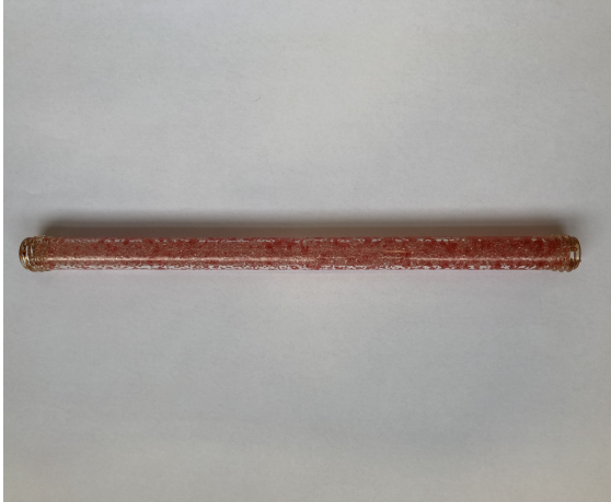
Figure 5.13: A darker color is observed at inlet and outlet of the bead pack. This is believed to be an accumulation of the red particles used to dye the EXXSOL D60.
