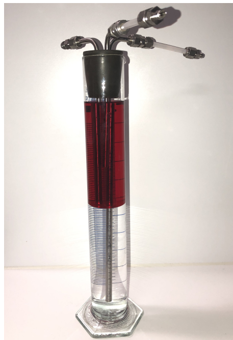
Figure 3.4: Oil-water reservoir. Inlet tubes placed in the center of their respective fluid columns, and outlet tube placed in the middle of the two phases.
