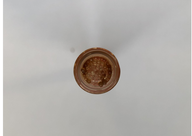
Figure 5.13: A darker color is observed at inlet and outlet of the bead pack. This is believed to be an accumulation of the red particles used to dye the EXXSOL D60.
