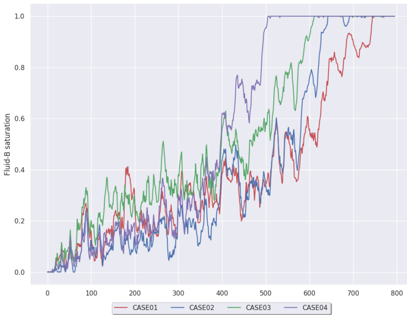
Figure 5.12: Averaged y -direction water saturation plot of CASE01, CASE02, CASE03, and CASE04. Lower viscosity oil advances further into the micromodel.
