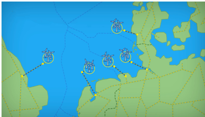
Figure 2.5: Point to point connections of offshore wind farms to shore [30].
