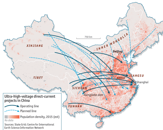
Figure 2.2: Planned and operating HVDC projects in China per 2017, connecting remote hydropower resources [20].
