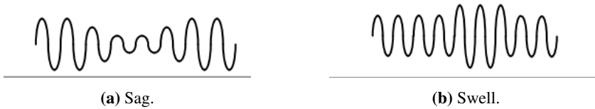
Figure 2.12: Example waveforms of sag/swell disturbances [36].
