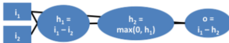
FIGURE 3.5: Network computing o = \min(i_1, i_2) , assume i_1 = i_2 = 0 , when i_1 < i_2 then \frac{dy}{di_2} = 0 and when i_2 < i_1 then \frac{dy}{di_1} = 0 . Using LRP or Integradient Gradients at this network would result in importance assigned exclusively to either i_1 or i_2 . With the RevealCancel rule, DeepLIFT assigns 0.5\min(i_1, i_2) attribution to both inputs [82].
