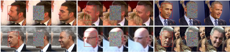
Figure 4.1: DeepPrivacy results on a diverse set of images. The left image is the original image annotated with the bounding box and keypoints, the middle image is the input image to our generative model, and the right image is the generated image. Note that our generator never sees any privacy-sensitive information.
