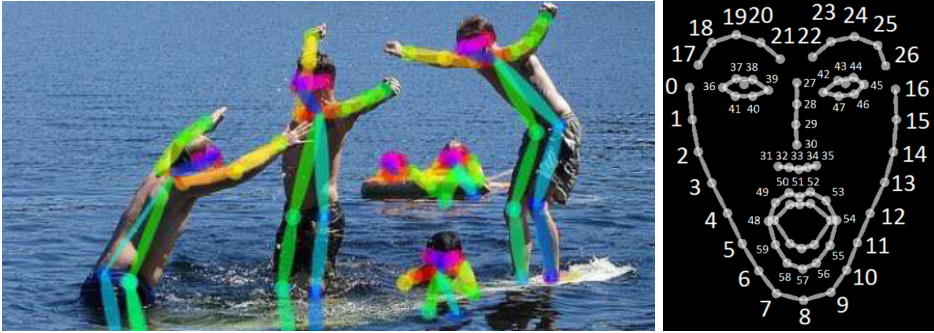
Figure 2.2: OpenPose Predictions Left : Examples of predicted poses from OpenPose. Right : Face keypoints that OpenPose predicts. Figure source: https://github.com/CMU-Perceptual-Computing-Lab/openpose
