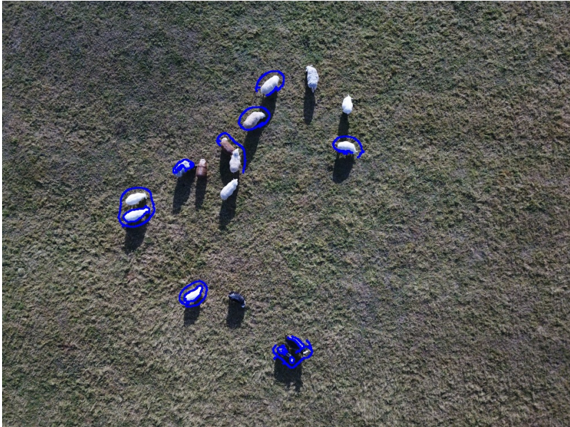
(b) Contours found in the image in Figure 3.1 after applying the Bilateral Filter and removing the shadows.
