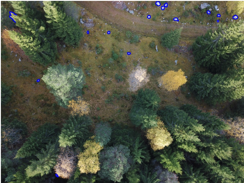
(b) Example of false positives found when using Dilation with Bilateral Filter. We can see that a lot of irrelevant objects, mostly rocks, are detected.
