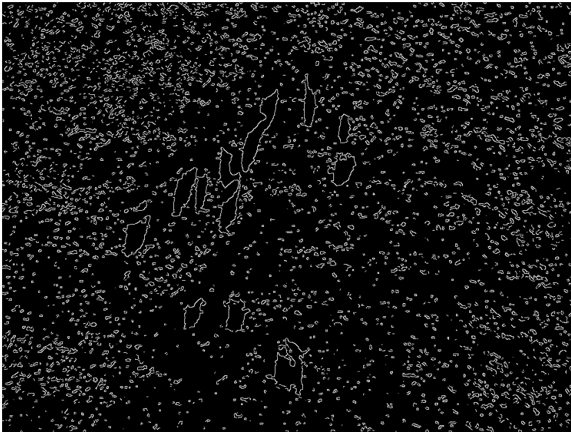
(b) Edges found in image with Truncated Thresholding applied to Gaussian filtered grayscale image.
