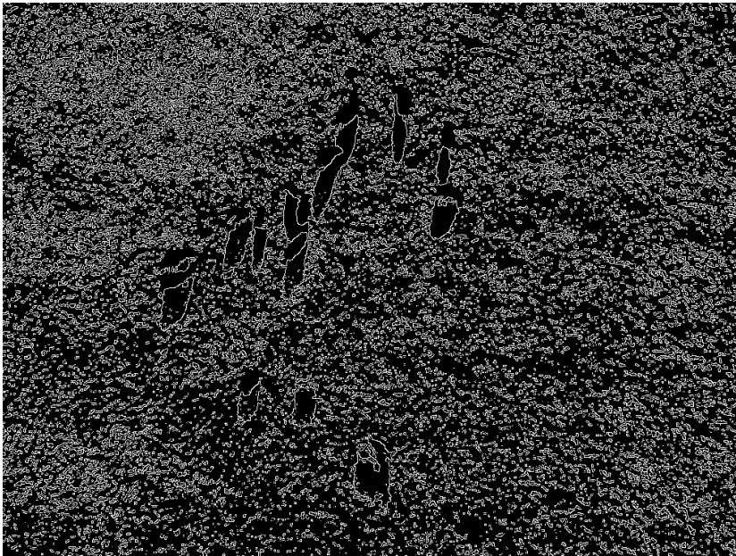
(b) Edges found in image with Truncated Thresholding applied to grayscale image.
