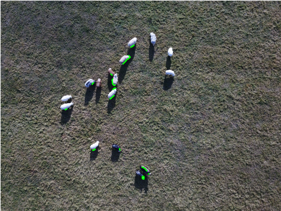
Figure 3.12: Contours found in image with Truncated Thresholding applied to Bilateral filtered grayscale image. Good results after finding contours, the solution found all the black sheep and one brown sheep.
