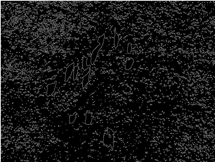
(b) Edges found in image with Binary Thresholding applied to Gaussian filtered grayscale image.
