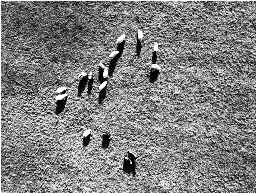
(b) Histogram Equalization applied to the image in Figure 3.1 after converting it to grayscale.
