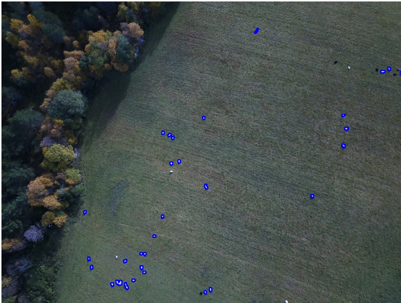
(a) Example of sheep detected when using Dilation with Bilateral Filter. As we can see, most white sheep are detected, but it has problems detecting black sheep.
