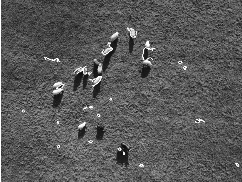
(b) Contours found in the image in Figure 3.1 after converting it to grayscale and applying the Bilateral Filter and Histogram Equalization.
