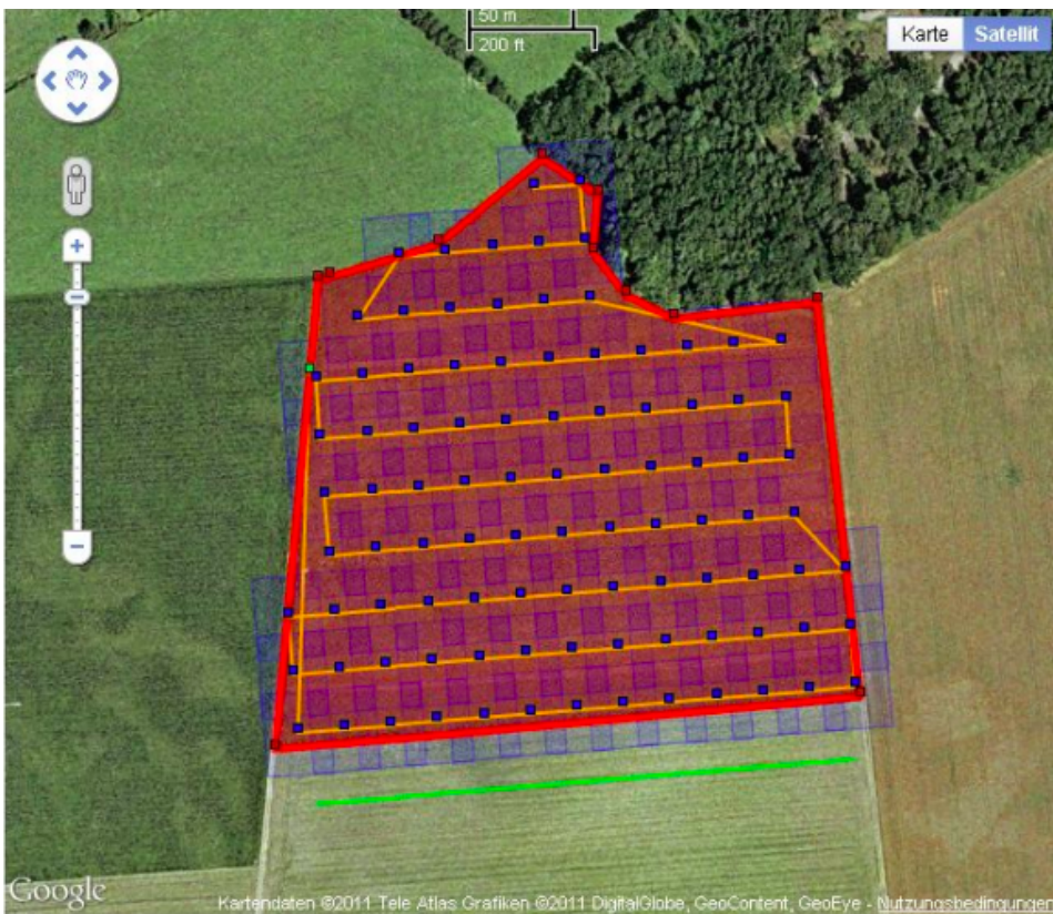
Figure 5.1: Waypoint Editor[21]. With the use of Google Maps Application Programming Interface, they developed a program that allowed them to mark the area they wanted to search with the UAV.
