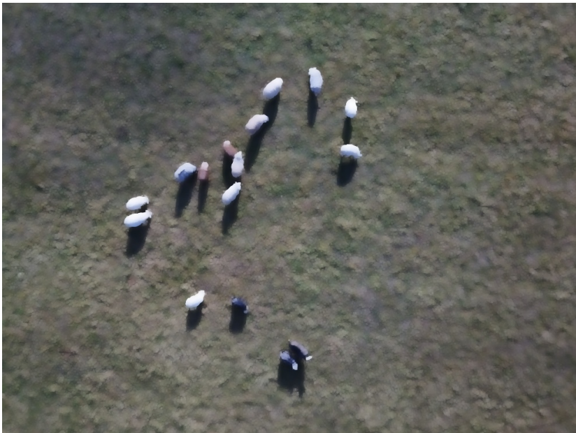
(b) The result of applying both Dilation and Bilateral Filter to the original image. It makes the objects appear bigger as well as smoothing the background.
