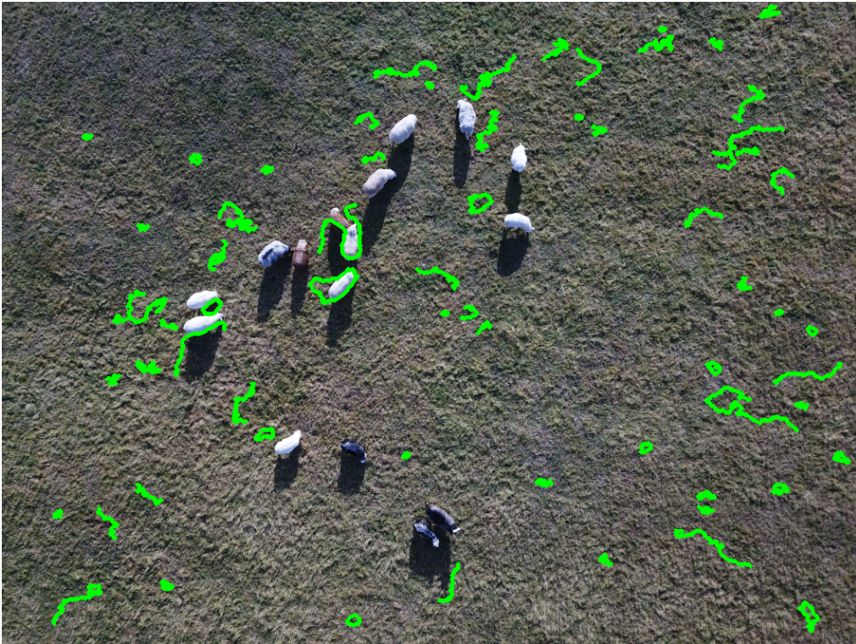
Figure 3.21: Contours found in image with Otsu Segmentation applied to Bilateral filtered grayscale image. It does not find any black sheep, and there are many false positives.
