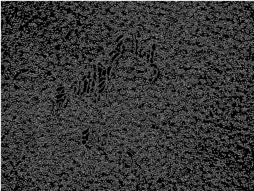
(b) Edges found in image with Adaptive Mean Thresholding applied to Bilateral filtered grayscale image.
