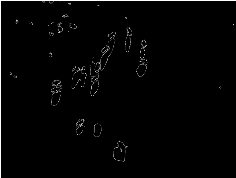
(b) Edges found in image with Threshold To Zero method applied to Bilateral filtered grayscale image.
