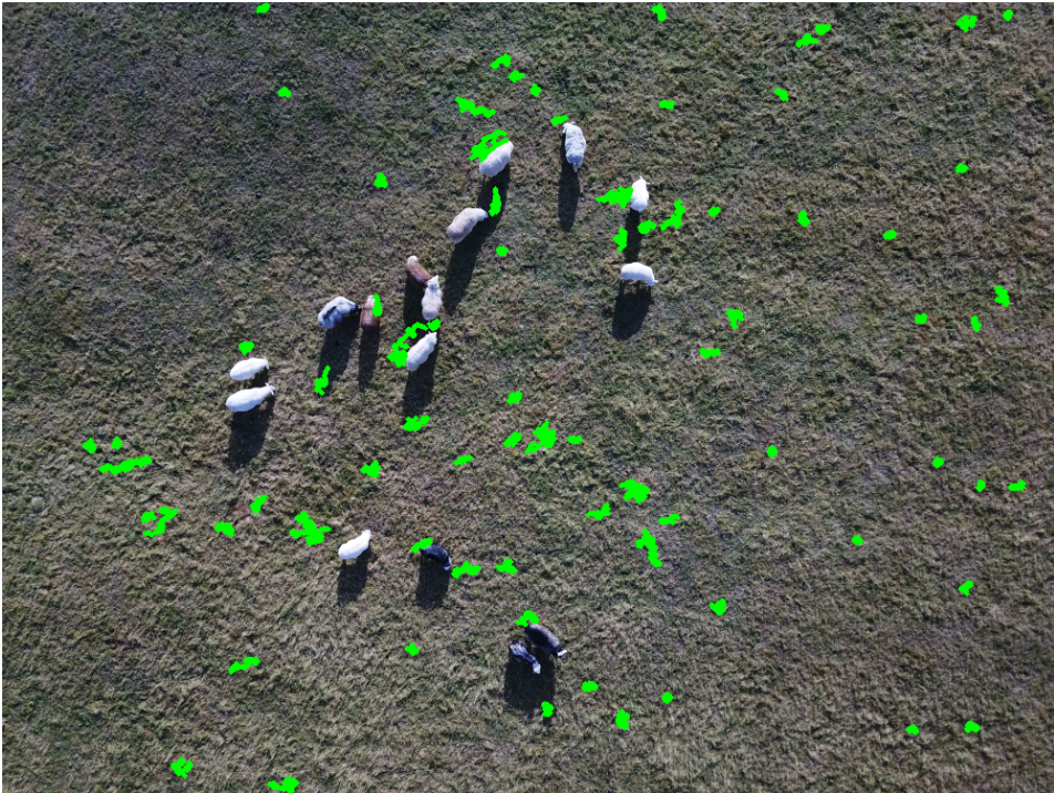
Figure 3.29: Contours found in image with Adaptive Mean Thresholding applied to Bilateral filtered grayscale image. It finds some of the black sheep, but also many false positives.
