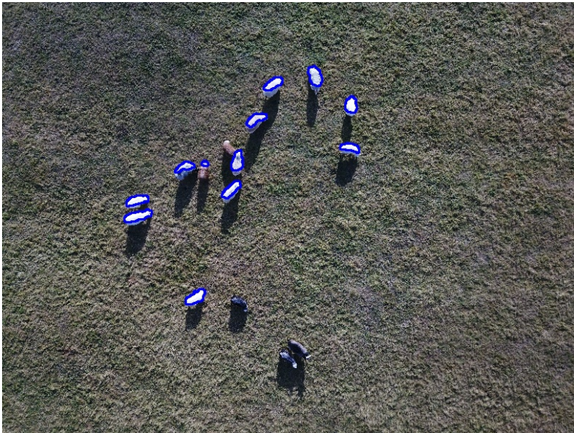
(b) Contours found using the method of removing all other colors than the desired one, drawn on the original image. As we can see are all the white sheep detected in this image.
