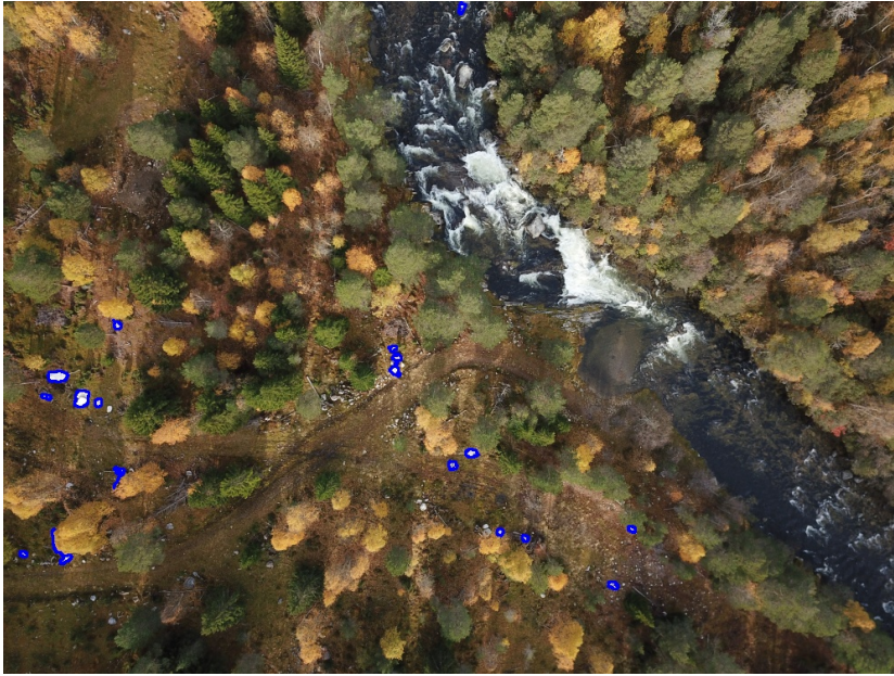
(a) Example of falsely detected objects using the Solution using Dilation with Bilateral Filter .
