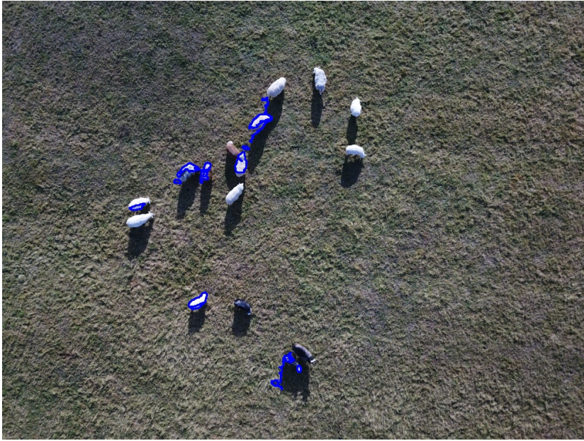
(a) Contours found in the image after applying the Meanshift Filter to the image in Figure 3.1 .
