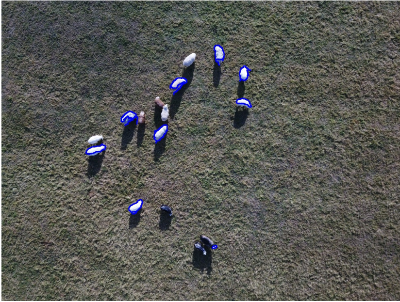
(a) Contours found in the image in Figure 3.1 after applying the Bilateral Filter and Dilation.
