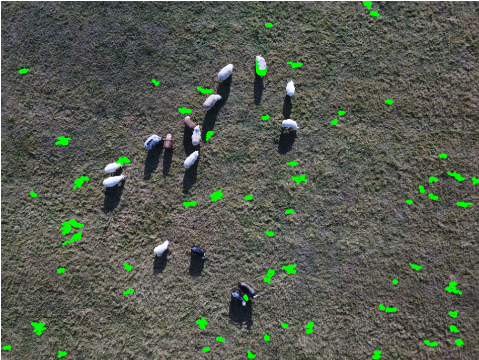
Figure 3.25: Contours found in image with Adaptive Mean Thresholding applied to Bilateral filtered grayscale image. It does find one black sheep, but also many false positives.
