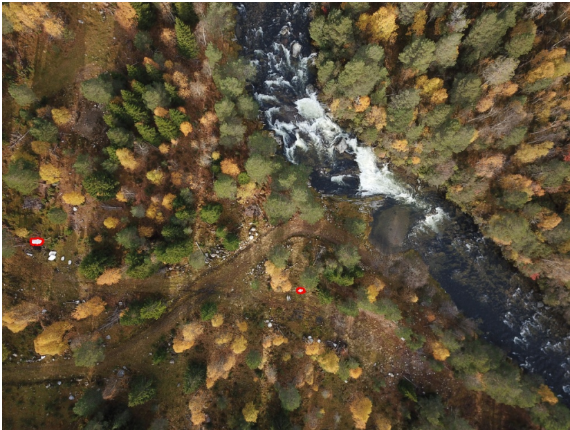
(b) Example of falsely detected objects after adding the Bounding Rectangle to the Solution using Dilation with Bilateral Filter .
