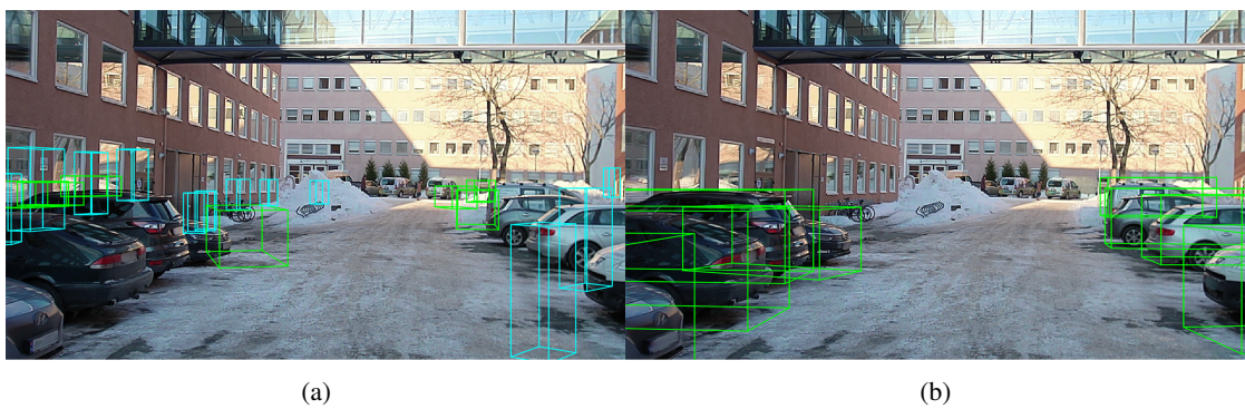
Figure 5.30: SECOND inference on NAP sample 140 without (a) and with (b) pre-training on CADET.
