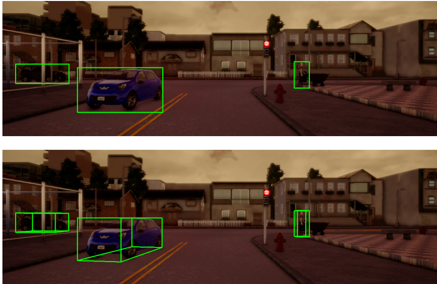
Fig. 2: 2D (top) and 3D (bottom) bounding boxes as generated by CADET. Class labels are omitted.
