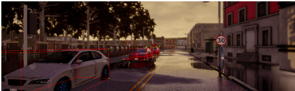
Figure 5.4: Vertex occlusion detection. Occluded vertices are shown in red, while visible vertices are shown in green.
