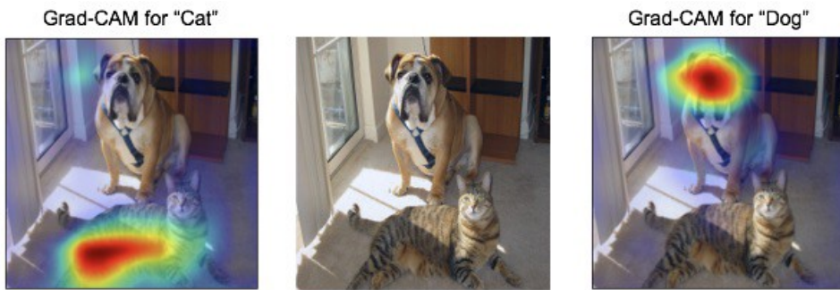
Figure 4.2: An illustration of what GradCAM can show. Here a convolutional net is trained to distinguish cats from dogs, and the tool illustrates which features were important for the classifier to determine that the image consisted of a dog or a cat. From the activations, one can see that the face of the boxer was significant, and probably a distinguishing feature between the cats and the dogs the classifier noticed in the training set. The cat has very high activation on the belly, probably due to the stripes being a distinguishing feature. Figure courtesy of Selvaraju et al. (2016).
