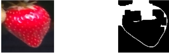
Figure 2.3: Strawberry before (left) and after (right) filtering, Canny edge detection and closing.
