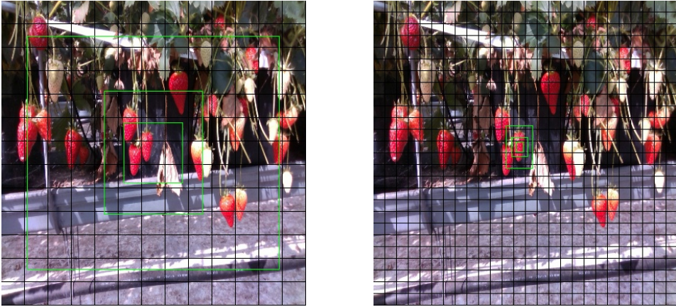
Figure 2.20: Detection on a grid cell with YOLOv3-tiny at first (left) and second (right) scale with three bounding boxes per scale.
