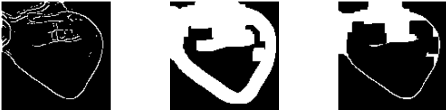
Figure 2.8: Result of hysteresis (left), result of dilation of hysteresis (middle) and result of closing, or erosion of dilation (right).
