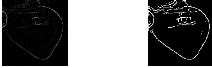
Figure 2.7: Result from non maximum suppression before (left) and after (right) double threshold application and tracking by hysteresis.
