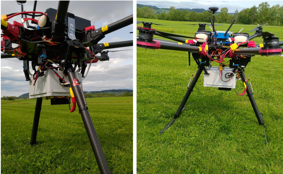
Figure 5.12: Mounting of payload to multirotor
