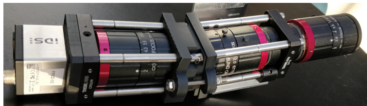
Figure 4.1: Engineering model of HSI camera. The gray box to the very left is a CMOS image sensor from iDS. The optical parts include lenses and a diffraction grating from Edmund Optics , and adaptors, mounting parts and a slit from Thorlabs [5].
