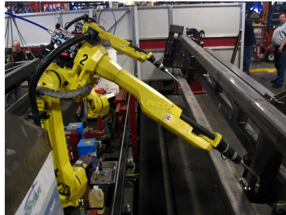
Figure 1.2: A set of six-axis robots used for welding. Picture Wikipedia
