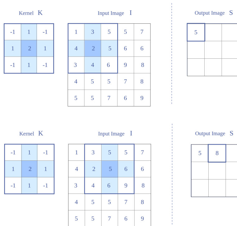
Figure 2.5: An illustrated example of two steps of the convolution of a kernel, K , and an image, I . The convolution in this example is performed with a stride of 1 and without padding the image.
