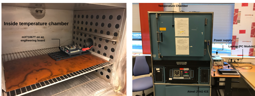
Figure 7.2: Photo of the test setup used at 105^{\circ}C . Right is outside the chamber, left is inside the chamber.
