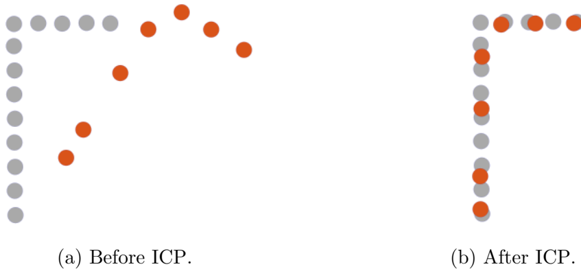
Figure 5.4: Two point clouds being matched using ICP. The gray dots are point in the model \mathbf{X} , and the orange points are in the measured data points \mathbf{P} .
