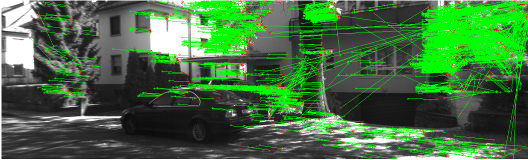
(a) Image showing the features tracked from frame 1952 to frame 1953 in the KITTI dataset. Screenshot taken from the best of the six tests.
