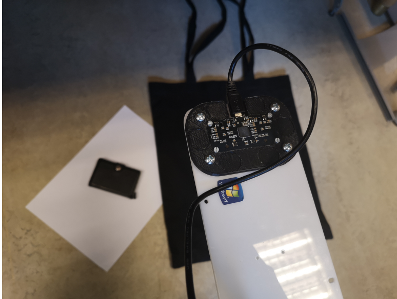
Figure 23: Image showing the camera facing downwards towards the floor, where contrasting objects are placed to ensure good keypoint detection.
