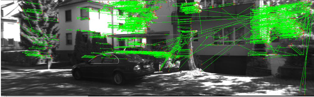
(a) Image showing the features tracked from frame 1952 to frame 1953 in the KITTI dataset. Screenshot taken from the best of the six tests.
