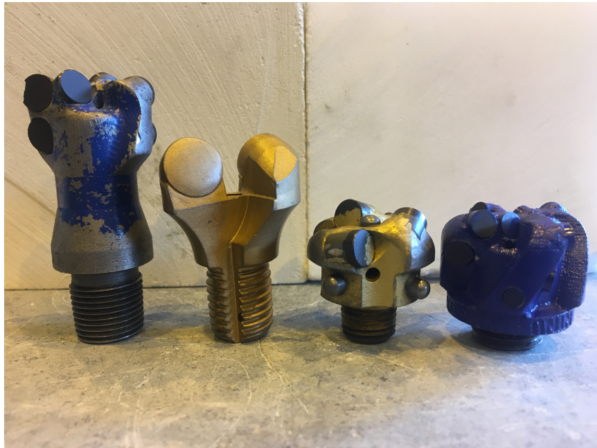
Figure 23: Drillbits. From left to right: NTNU 2018 custom bit, Alibaba bit, DSATS bit and NTNU 2019 custom bit.
