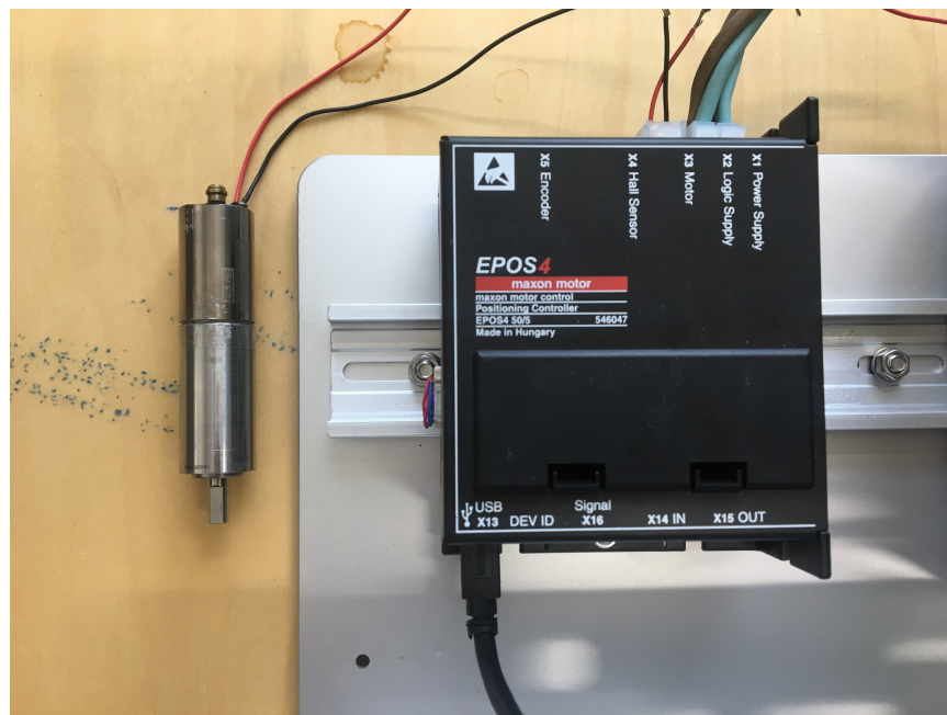
Figure 22: Maxon DCX19S motor and EPOS4 motor drive.
