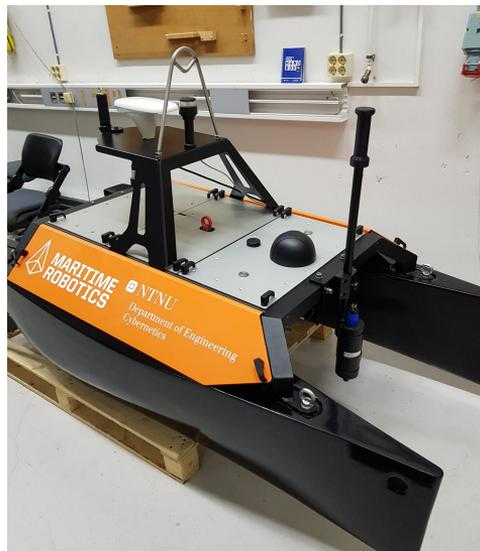
**Figure 1.1:** USV Otter with mounted hydrophone
