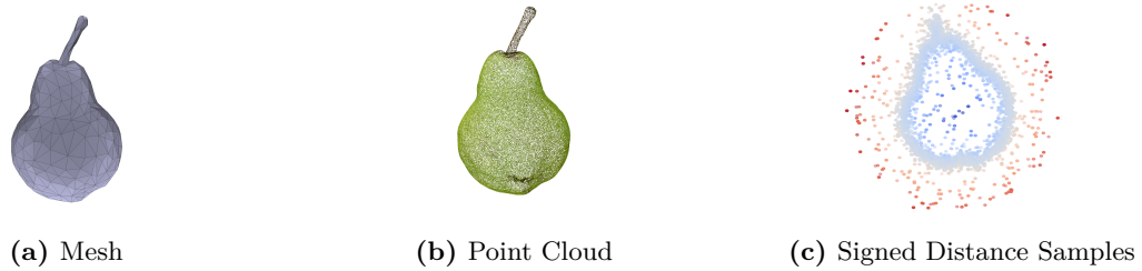
Figure 4.3: Example object in the custom-made 3D object set consisting of fruit and vegetables, processed food, and an assortment of bread. Left: A subsampled mesh with the color information removed. Middle: A point cloud generated from the mesh using Poisson disk sampling. Right: Signed distance samples generated by perturbing the point cloud with Gaussian noise, calculating the distance to the unperturbed points, and finally finding the sign of the distance by registering whether the perturbed points are inside or outside the mesh.
