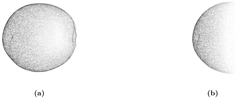
Figure 1.2: Left: A complete point cloud of an orange. Right: A partial point cloud of an orange, which would be what a camera system would see if it was viewing the orange from the left side of the image. The color information has been removed and replaced by a grayscale map to better illustrate the depth as seen from the camera.
