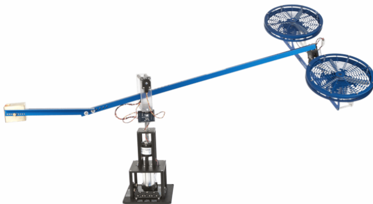
Figure 2.1: Quanser's 3 DOF helicopter
