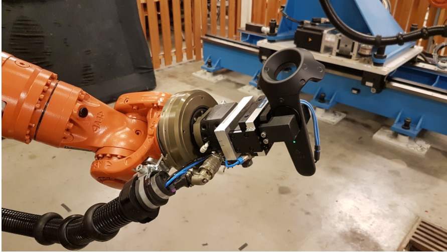
Figure 5.4: Vive controller firmly attached to the robot's gripper.
