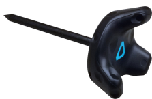
Fig. 8. Simple tool based on an HTC Vive Tracker with a 15 cm long and 1 cm thick spike probe screwed into its quarter inch UNC threaded camera mount.
