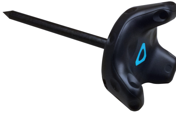
Figure 7.6: Calibration tool based on a Vive tracker with a 15 cm long and 1 cm thick spike probe screwed into its ¼" UNC threaded camera mount.
