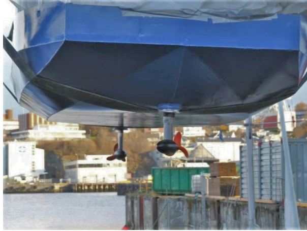
Figure 2.3: Two azimuth thruster located fore and aft on the milliAmpere ferry. Courtesy of Egil Eide, NTNU.
