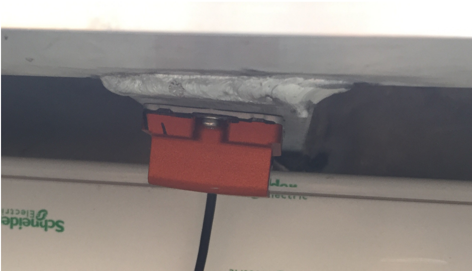
Figure 7.3: The mounting of the IMU. The sensor has a slight offset in negative roll.
