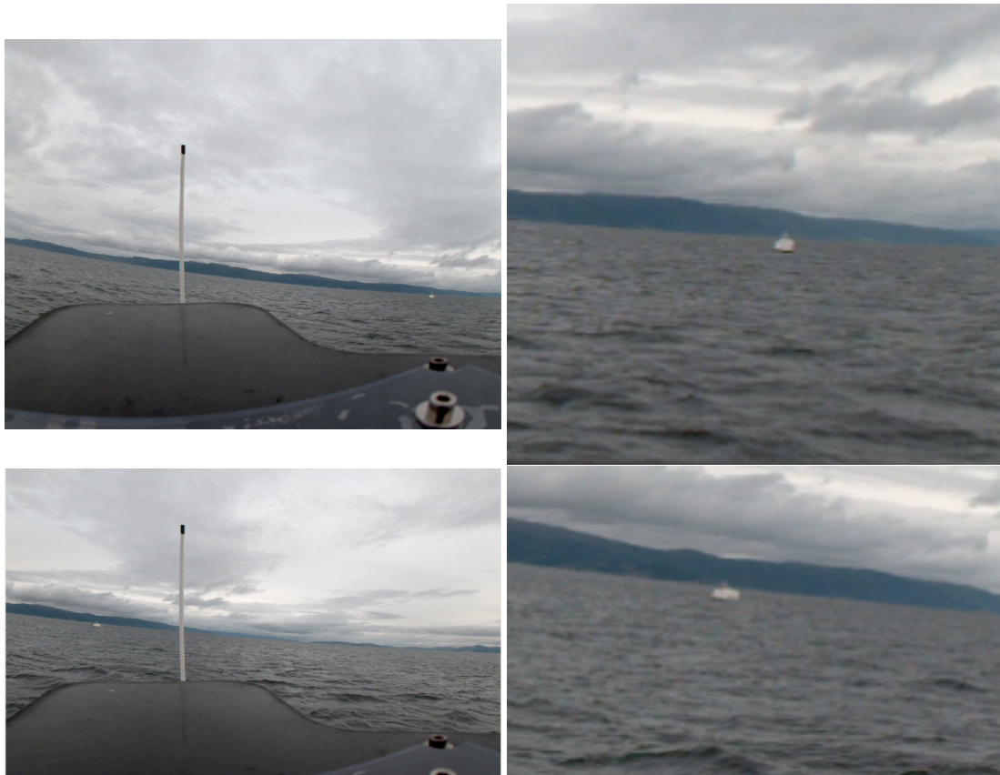
Figure 6.4: Examples of the performance of the YOLOv3 detector on the raw Ladybug images. The target vessel "Ocean Space Drone 1" is too far away and too small to be detected
