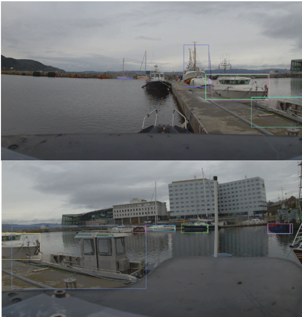
Figure 6.8: Examples of the multi-target performance of the combined YOLOv3-tiny detector and the Re^3 tracker. The pruning of old tracks is not optimized.
