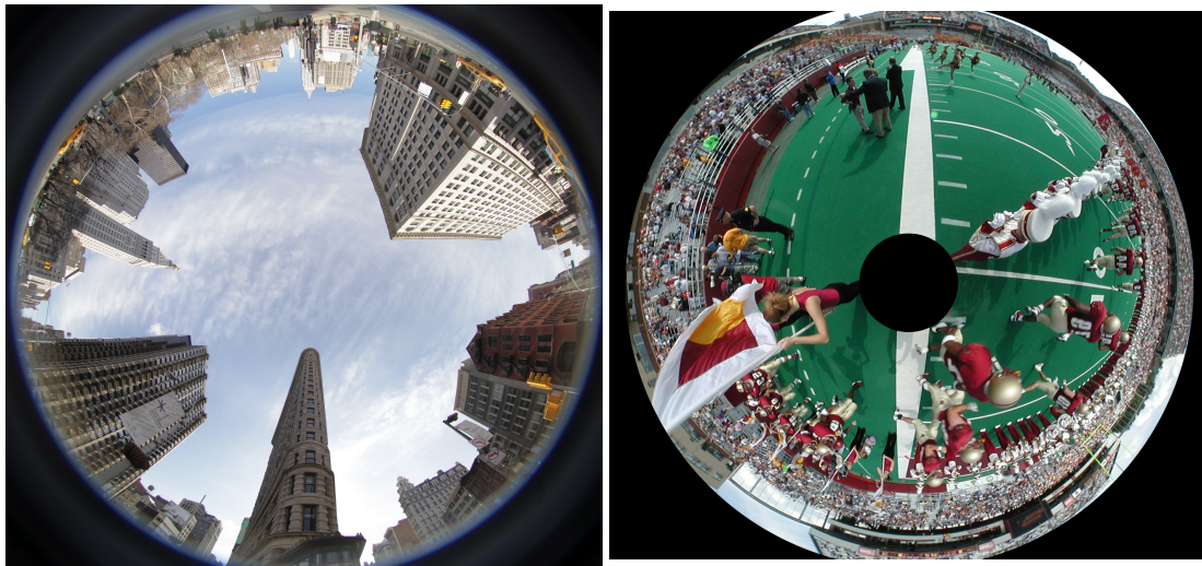
Figure 2.4: Fisheye camera and hyperbolic mirror camera compared. Wikimedia Commons and Columbia University CAVE project.
