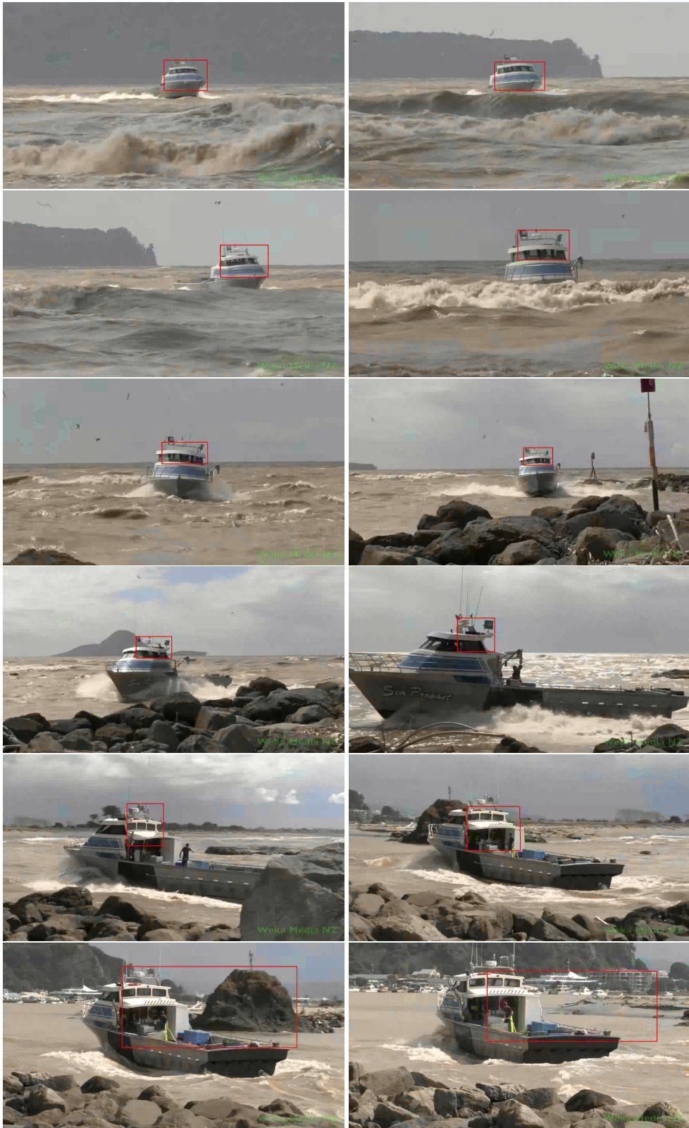
Figure A.8: Examples of the tracking performance of the Re^3 tracker. The tracker was initialized manually with a bounding box containing the boat. Video from YouTube: Weka Digital Media NZ
