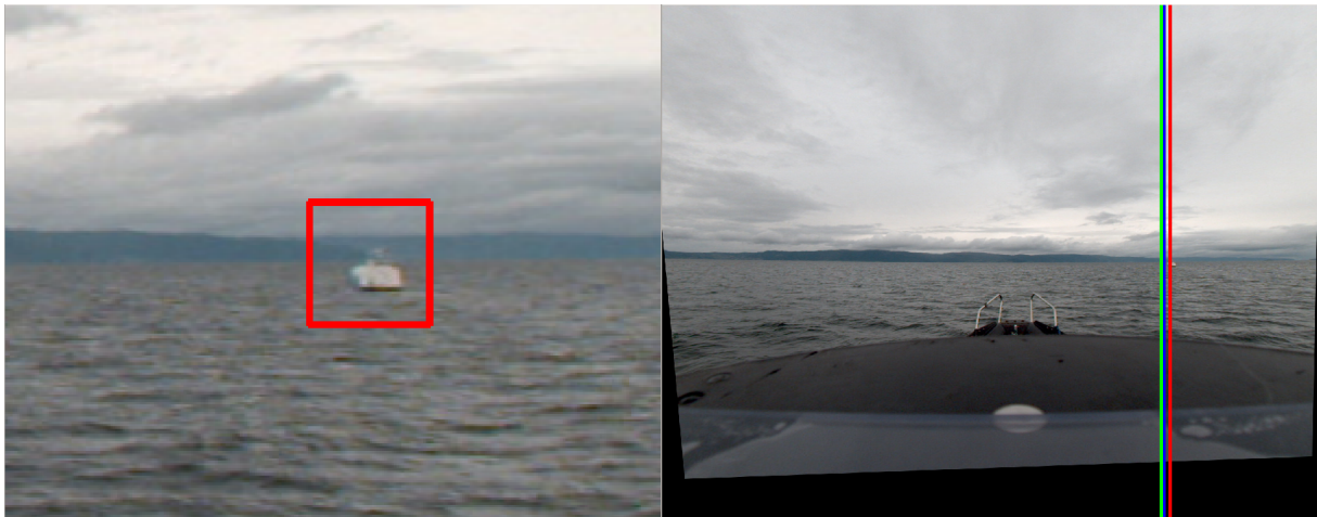
Figure 6.9: Target tracked using Re^3 in left image. In the image on the right the vertical lines indicate estimated position by the EKF (blue), RADAR detection (red), and camera detection (green). Slight delay might be visible. Test 1
