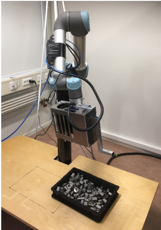
Figure 1.1: Photo of the robot cell at SINTEF Digital Trondheim. Notice especially the camera housing with the L-shaped gripper attached. Photo courtesy of Katrine Seel, MSc, SINTEF Digital.
