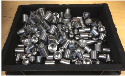
Figure 1.2: Cylindrical objects to be picked from plastic bin covered with felt. Photo courtesy of Katrine Seel, MSc, SINTEF Digital
