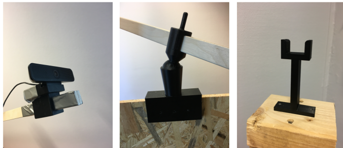
Figure 4.4: The 3D printed objects. The attachment between the camera and stick(left). Attachment between stick and test wall(middle). The docking of the stick(right).
