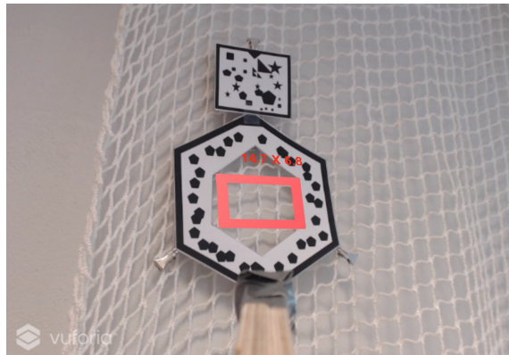
Figure 3.14: The outline of hole with size during testing. The red outline indicates that a marker with net of color red have to be attached to fix the hole.
