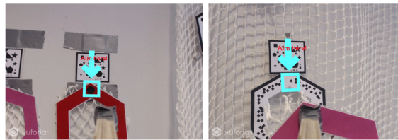
Figure 3.16: The "Aim here!" indicator is shown both when the stick is attached to the marker with net(left), and when that marker is attached to the AR marker to fix the hole temporarily(right).
