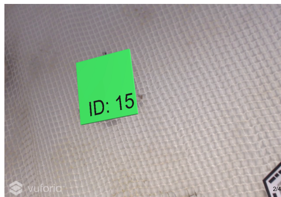
Figure 3.2: The ID board shown during testing. The bright colors of the ID board make it easy locating where the hole is.
