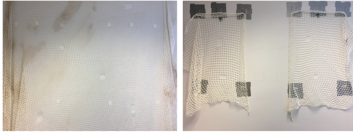
Figure 4.5: The plain test scenes with only the fish cage nets with holes. During testing, additionally AR markers and other components will be part of the test scenes. The plain test scene of the INFO experiment(left), and the plain test scene of the INTERACTION experiment(right) are shown.
