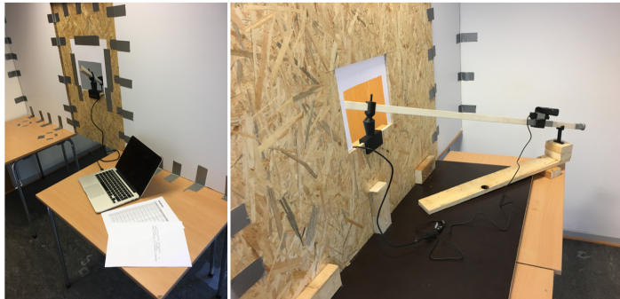
Figure 4.2: In front of the test wall(left) with the workstation in the front. Behind the test wall(right) with the stick, with a camera attached, placed in the docking.
