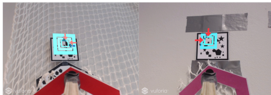
Figure 3.19: If several adjustments have to be done, multiple correction arrows appear to correct the path.
