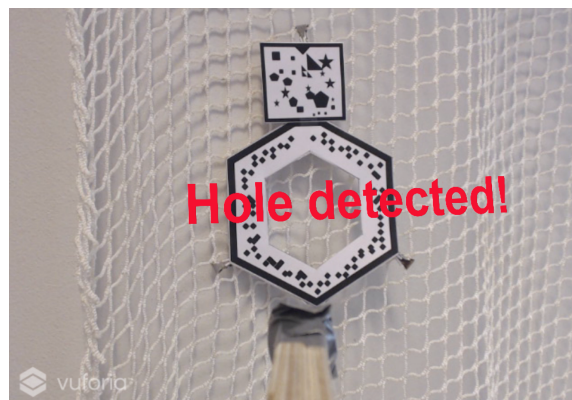
Figure 3.12: The "Hole detected!" alert presented during testing of the AR system. The indication is easy to discover, and has high readability.
