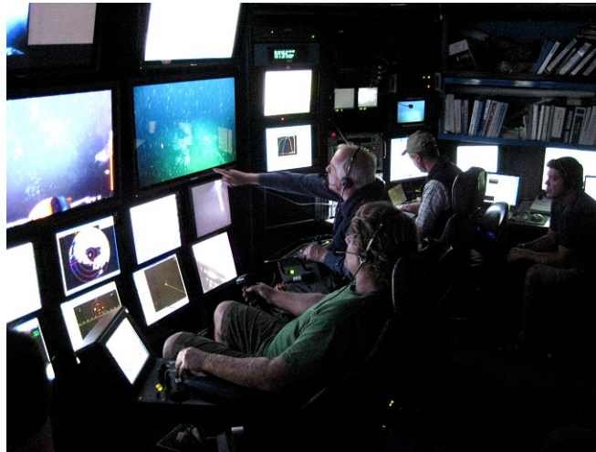
Figure 5.18: The operating room of multiple subsea ROVs, illustrates how the operators have different screens with information to backup the main video feed from the ROV. Source [126].
