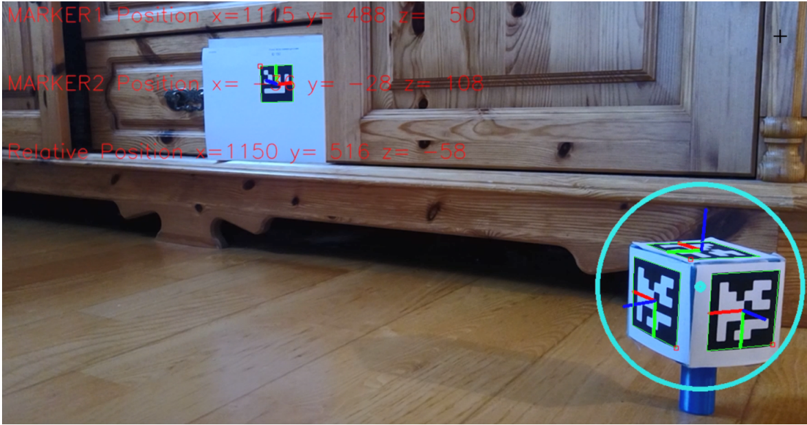
Figure 3.3: The developed OpenCV program which tracks multiple ArUco markers, both 2D and the developed 3D marker.
