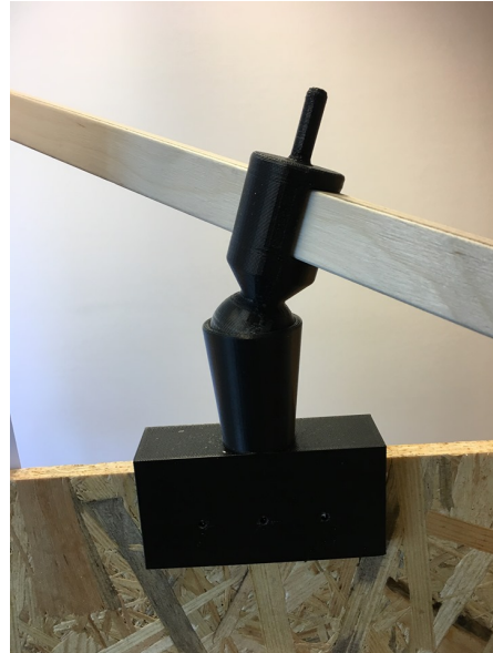
Figure 4.7: The ball joint mount used to control and operate the tool.
