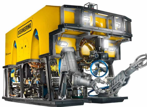
Figure 2.7: A work class ROV from Oceaneering [35] (the Millennium Plus), with the basic left manipulator and the more advanced right one.
