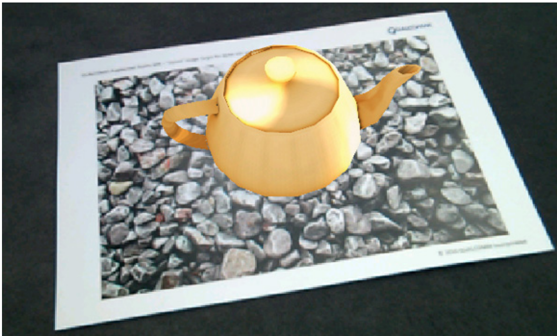
Figure 3.2: An image uploaded to the Vuforia database, which then acts as an image target (marker) with an added AR object on top of it. Source: [69].
