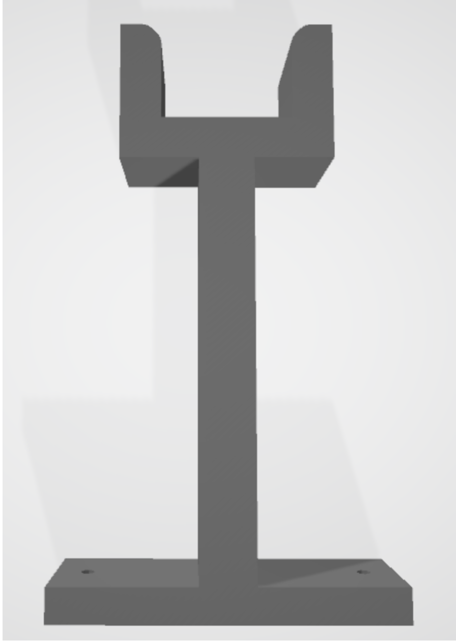
Figure B.8: A 3D model of the 3D printed docking used to enable the tool to be docked in between operations and during operation 3.
