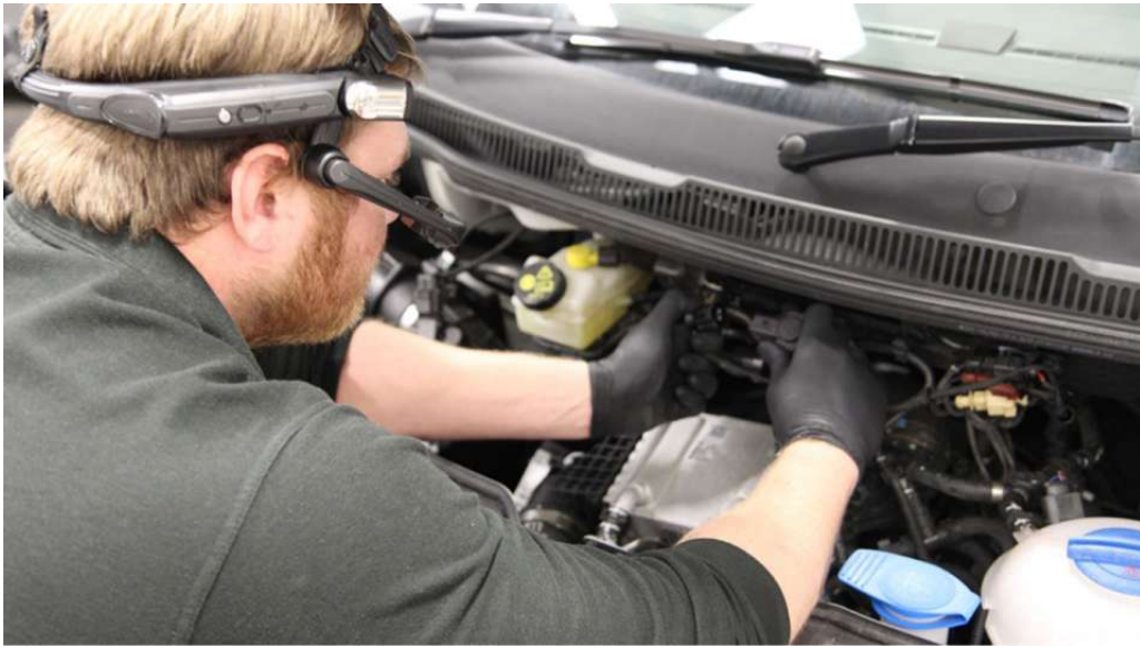
Figure 2.5: An operator using a head-mounted AR headset to see the AR visualization of the manual instructions during maintenance. Source: [28].
