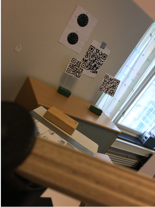
Figure 4.18: Operation 3 experiment scene, with the valves mounted on the wall used in the non-AR part, the standing markers are valves in the AR system and the wall mounted marker is a reference for the dialog boxes.
