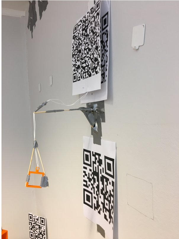
Figure 4.15: The operation 2 scene, with the quadratic hook placed on fragile wall mount.
