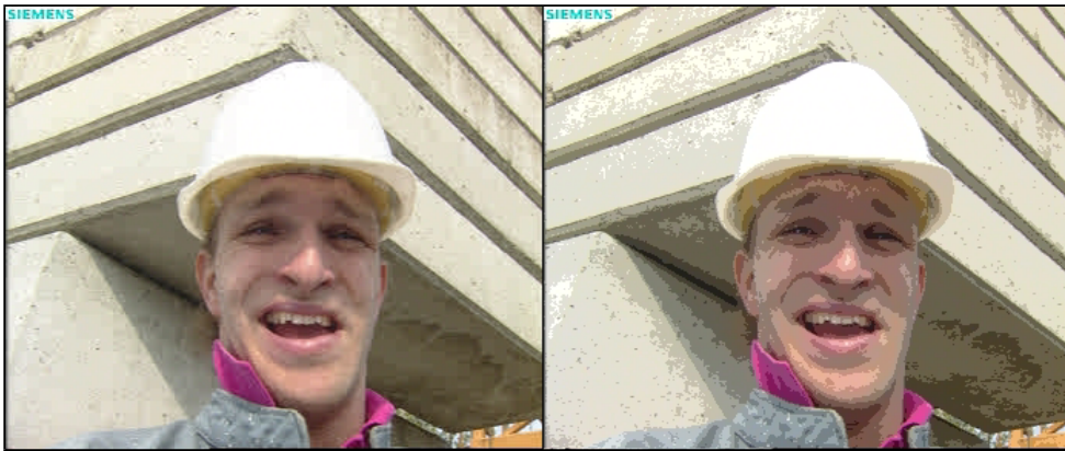
Figure 4.3: Comparison of the two custom coders using a natural video source. The left image is coded using the traditional coder. The right image is coded using the RSQ coder.
