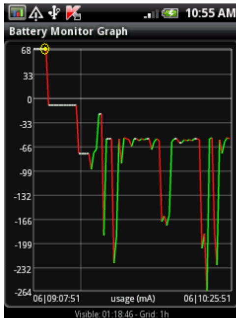
Figure 20: Battery current in mA vs. time for Kaspersky anti-virus
