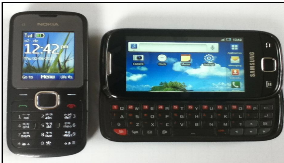
Figure 1: Comparison between a traditional mobile phone and a smartphone
