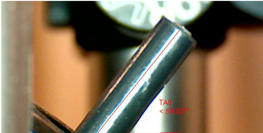
Figure 6.6: The angle of the fibre between the crystal and the detector in the ATR setup was found to be 50.827^\circ .
