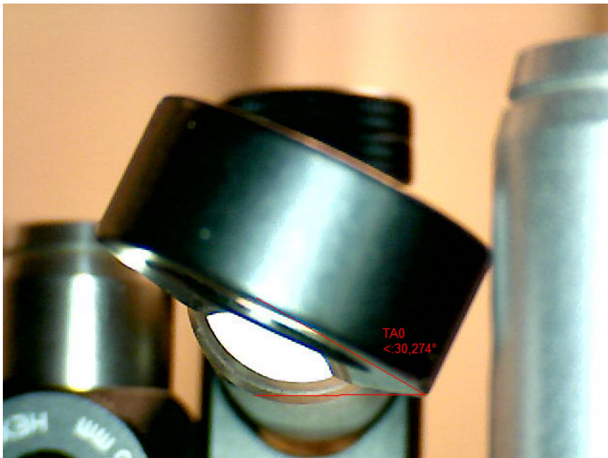
Figure 6.7: The angle of the lens between the crystal and the fibre leading the light to the detector in the ATR setup was found to be 30.274^\circ ..
