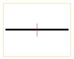
**Figure 4.4:** Illustration of the structure created when calculating the bands for a slab waveguide. The Red line illustrates the computational cell, in this case two-dimensional. The Master Equation is solved for wavevectors along the line defect. Same as for the line defect in Figure 4.3.
