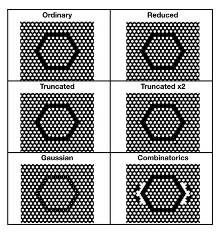
Figure 6.1: Two-dimensional illustration of the different ring resonator designs.
