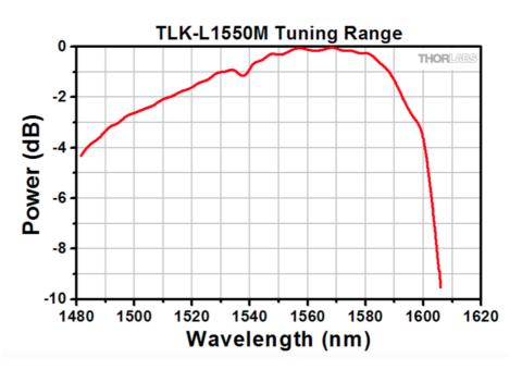
Figure 6.5: Power spectrum of the TLK-L1550M from Thor Labs.
