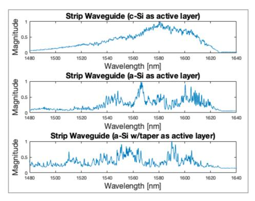
**Figure 5.20:** Transmission spectra for strip waveguides. The top spectrum represents the case where c-Si is the active layer. The middle spectrum represents the case where a-Si is the active layer. The bottom spectrum illustrates the case where a-Si with inverted tapers is the active layer. All spectra are normalized to unity.
