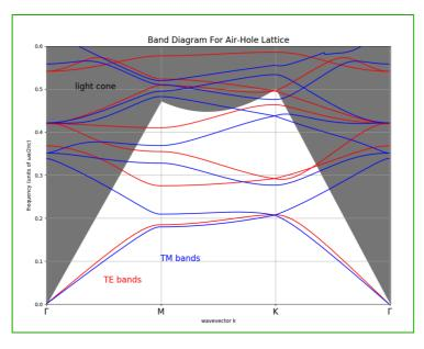
**Figure 2.12:** Band diagram for a hexagonal symmetric photonic crystal including the light cone. The TE and TM bands are shifted in frequency compared to Figure 2.11. The shift is caused by a difference in air-hole radius (air hole radius in Figure 2.11 is 0.48a while in this figure it is 0.3a). Frequency is given in units of  $\omega a/2\pi c$  and wavevector k is given in units of  $2\pi a/\lambda$ .
