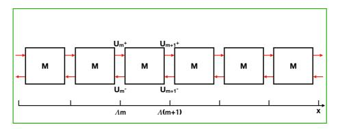
**Figure 2.5:** The x-axis is showing the periodicity  $\Lambda$  and the matrices above depict schematically equation 2.39. The propagation matrices must be added where the red-arrows are. **E**- and **H**-fields are represented by the potential function U here [55].
