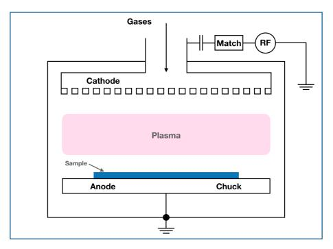
**Figure 3.3:** Cross-sectional illustration of a PECVD chamber. A combination of gases enters from the top and flows through a perforated metal sheet that acts as a cathode for the radio frequency source. When the gases are localized between the cathode and anode the radio frequency electric field interacts with the gases creating a plasma. The sample is placed on top of the chuck.
