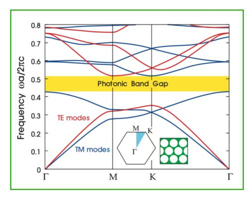
**Figure 2.11:** The yellow area is illustrating a complete photonic band-gap (for all polarizations). The white hexagonal structure centered in the bottom of the figure is the first Brillouin zone, and the blue triangle inside of it is the irreducible Brillouin zone. The horizontal axis is tracing the lines of high symmetry and the vertical axis is normalized frequency. The frequency is normalized with respect to the lattice constant *a* and speed of light, c (reprinted from [31]).
