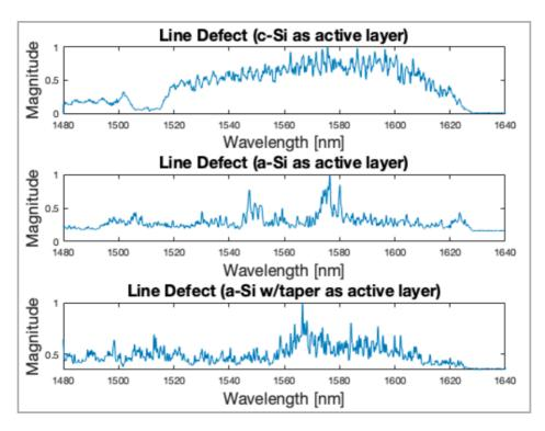
**Figure 5.21:** Transmission spectra for line defects. The top spectrum represents the case where c-Si is the active layer. The middle spectrum represents the case where a-Si is the active layer. The bottom spectrum illustrates the case where a-Si with inverted tapers is the active layer. All spectra are normalized to unity.
