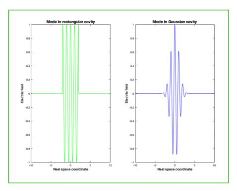
**Figure 2.15:** Plot illustrating a mode trapped in a rectangular cavity (green/left) and a mode trapped in a Gaussian cavity (blue/right).
