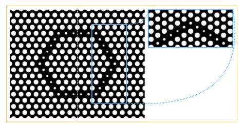
**Figure 5.1:** Figure describing the relation between the PCRRs and the illustrations in Table 5.1. The Gaussian design is used for illustration purposes. For all design solutions except for the combinatorics design the relation is as illustrates by the Gaussian design. The combinatorics design exhibits two-fold rotational symmetry, or mirror symmetry along the grey dashed line. All other designs exhibit the same six-fold rotational symmetry as the Gaussian design (see Appendix D).
