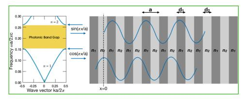
**Figure 2.7:** Illustration of how degenerate modes concentrate differently within a one-dimensional PC and how it results in a band-gap in frequency.
