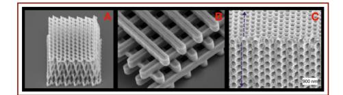
**Figure 1.2:** Pictures of an inverse Yablonovite (A), woodpile structure (B), and inverse spheres in a diamond lattice structure (C) all taken with a scanning electron microscope (reprinted from [59]).
