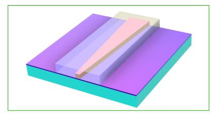
**Figure 2.19:** Illustration of an inverse taper waveguide. The waveguide is tapered from small to normal waveguide cross-section, opposite of traditional tapers. The waveguide is coated with a polymer material.
