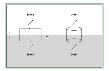
**Figure 2.1:** Depiction of how the tangential components of fields and normal components of fluxes behave at a boundary. Tangential components of **E**- and **H**-fields and normal components of **D**- and **B**-fluxes must be continuous across a boundary. In agreement with equations 2.29-2.32.
