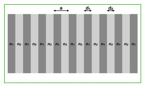
Figure 2.3: A stacked material with alternating refractive index  $n_1$  and  $n_2$ . *a* marks the periodicity and lattice constant of the structure,  $d_1$  and  $d_2$  indicates the distribution of the two materials.
