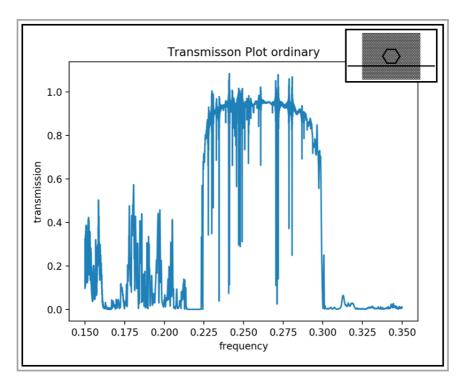
**Figure 5.9:** Transmission spectra for the design solution ordinary. Transmission spectra is normalized by the reference structure (see Figure 4.5). The transmission band is clearly visible from 0.225 to 0.300 normalized frequency. The transmission spectra exhibit several missing modes in the transmission band, assumed to have coupled to the ring resonator.
