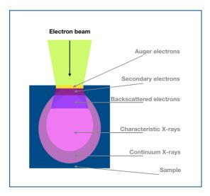
Figure 3.10: Illustration of the different electron/sample interactions and their interaction volumes.
