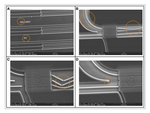
**Figure 5.16:** SEM images illustrating a case of badly performed development. Figure **A** is a macroscopic image showing exposed and developed ordinary and rm designs. Figures **B**, **C**, and **D** illustrate a PCRR structure with coupling to PC waveguide and slab waveguide. All four images are captured from the same sample. Yellow circles are points of interest.
