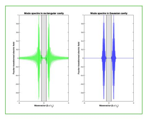
**Figure 2.16:** Spectra of the two trapped modes, rectangular cavity mode to the left and Gaussian cavity to the right. The gray area centered around a wavevector equal to zero defines leaky modes within the light cone. The rectangular cavity modes clearly exhibits more small frequency components, potentially leaking out into a surrounding cladding.
