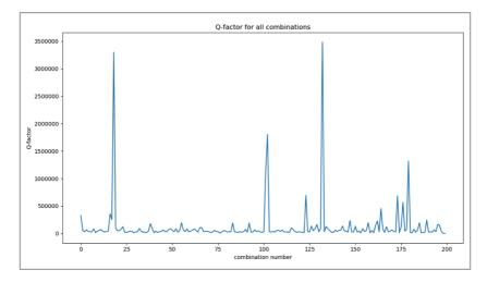
**Figure 5.2:** Result from the two-dimensional mode simulation on all 199 possible design solutions. Vertical axis is Q-factor and horizontal axis is design solution number. The peak q-factor value of  $3.5 \times 10^6$  belongs to design solution number 133.
