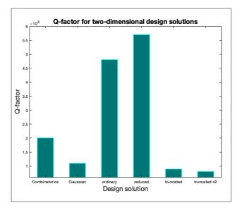
**Figure 5.12:** Diagram of Q-factors for all design solutions simulated in two-dimensions. All Design solutions exhibit Q-factor values of more than  $8 \times 10^7$ .
