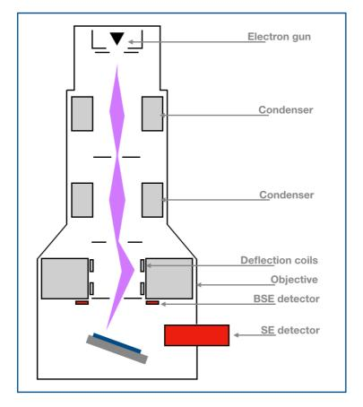
Figure 3.11 is a cross-sectional illustration of a SEM column.
