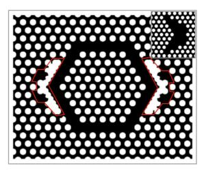
**Figure 5.3:** Illustration of the design solution achieving the highest q-factor (q-factor of  $3.5 \times 10^6$ ). The red areas defines the combinatorial computational cell. The inserted structure illustrates the structure used to distinguish the possible solutions by their q-factors.
