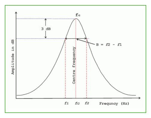
**Figure 2.17:** Illustration of how Q-factor is defined in frequency-space. The Q-factor increases with an increasing  $f_c$  and decreasing B.  $f_c$  is the center frequency of a mode, while B is the bandwidth of the mode at full-width-half-maximum (FWHM) (i.e. an amplitude reduction of 3 dB).
