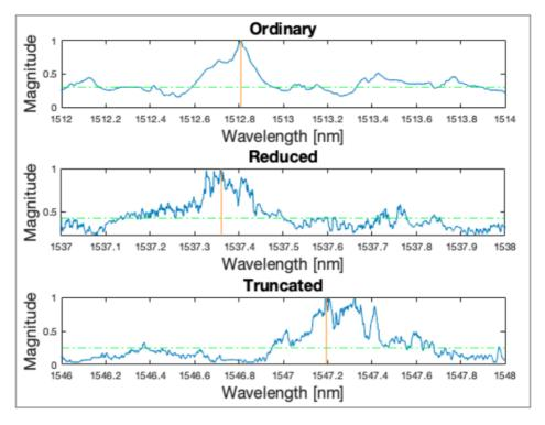
**Figure 5.22:** Transmission measurements focused in on most prominent frequency component for design solutions ordinary, reduced, and truncated. The wavelength resolution varies from spectrum to spectrum.
