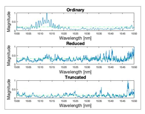
**Figure 6.6:** Transmission measurements for PCRR designs ordinary, reduced, and truncated over the wavelength range 1500-1550 nm. The green dashed line indicates the mean spectral value. All designs are produced in c-Si layer. Spectra are normalized to unity.
