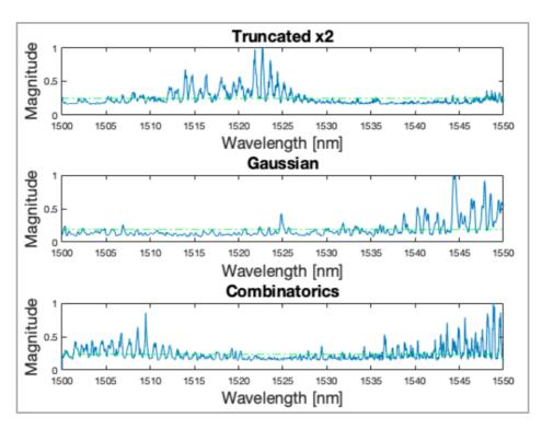
**Figure 6.7:** Transmission measurements for PCRR designs truncated x2, gaussian, and combinatorics over the wavelength range 1500-1550 nm. The green dashed line indicates the mean spectral value. All designs are produced in c-Si layer. Spectra are normalized to unity.
