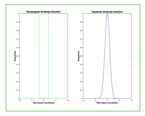
**Figure 2.14:** Plot illustrating the functions in table 2.1. Left graph illustrates the rectangular function, also stated mathematically in the top-left box of Table 2.1. Right graph illustrates the Gaussian function, also stated mathematically in the bottom-left box of Table 2.1. They mathematically illustrate the spatial constraints inflicted on a mode in a line defect (see Figure 3.4 for line defect).
