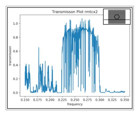
**Figure 5.10:** Transmission spectra for the design solution rmtcx2. Transmission spectra is normalized by the reference structure (see Figure 4.5). The transmission band is clearly visible from 0.225 to 0.300 normalized frequency. The transmission spectra exhibit several missing modes in the transmission band, assumed to have coupled to the ring resonator.
