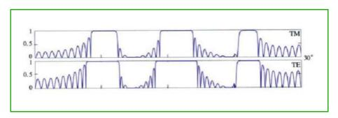
**Figure 2.6:** Transmission plot for an unknown one-dimensional crystal. The angle of incidence is  $30^{\circ}$ . The horizontal axis is normalized frequency. The transmission is dependent on polarization, as expected from Fresnel equations [55].
