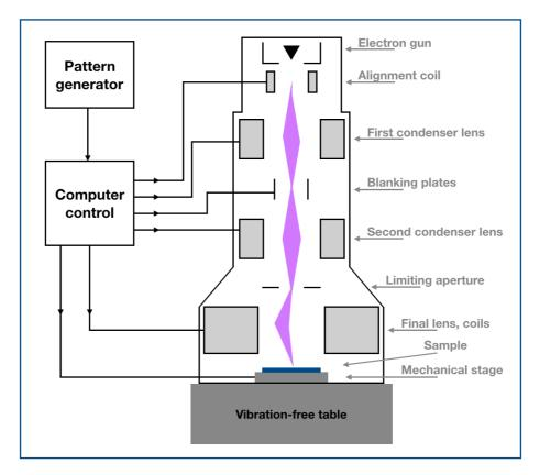
Figure 3.6 is a schematic cross-section of an EBL chamber with external connections to computer and pattern generator.
