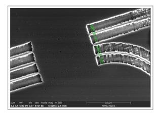
**Figure 5.15:** SEM-image of an etched and resist stripped sample. Approximate slab waveguide width is marked in green as 485.8 nm and 564.6 nm for the straight waveguide and curved waveguide, respectively. A PC structure is barely visible and the hole uniformity is poor.
