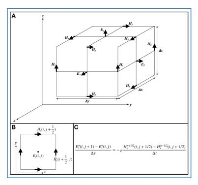
**Figure 3.2:** Illustration of a cubic Yee-cell (**A**), a two-dimensional Yee-cell (**B**), and how ME are calculated at the cell boundary (**C**). The Yee-cell is defined in FDTD Designer (see Figure 3.1), usually by the user in terms of dimension and resolution. The computation of ME as illustrated in Figures **A**, **B**, and **C** is a good description of steps "UPDATE H-FIELD" and "UPDATE E-FIELD" in the FDTD Simulator of Figure 3.1.
