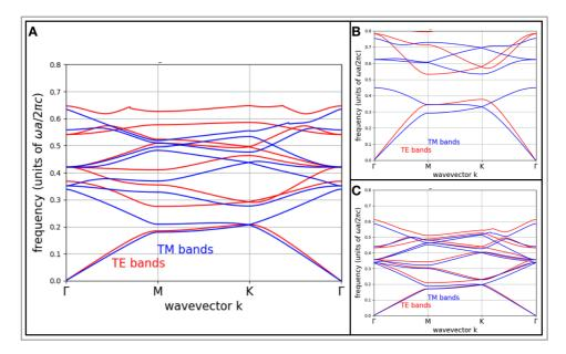
**Figure 5.4:** Band diagrams for two-dimensional triangular air-hole lattice PC with hole radii 0.3a (**A**), 0.48a (**B**), and 0.2a (**C**). As the hole radii is increased the dispersion relation blue-shifts in frequency. The band-gaps themselves increases with increasing hole radii.
