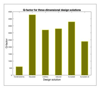
**Figure 5.13:** Diagram of Q-factors for all design solutions simulated in three-dimensions and with silica as substrate. All design solutions exhibit Q-factor values of more than 2000, except for the combinatorics design solution.
