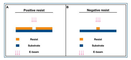
**Figure 3.5:** Illustration of the logical differences between positive (**A**) and negative (**B**) resist after development. Positive resist becomes more soluble when exposed to an electron beam. Negative resist becomes less soluble when exposed to an electron beam.
