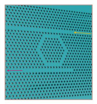
**Figure 1.3:** Three-dimensional illustration of the top silicon layer of a PCRR. Input and output waveguides are marked with a yellow and pink arrows, respectively.
