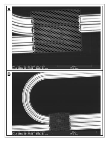
**Figure 5.17:** SEM-images illustrating the results of a well performed development process. SEM-images show no sign of resist cracks, waveguide bending, or waveguide cracking.
