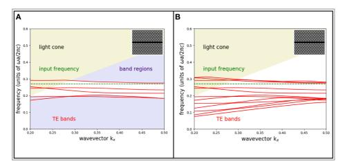
**Figure 5.5:** Dispersion relation along x-direction for line-defects in two-dimensional PC is illustrated in figures **A** and **B**. Input frequency is illustrated with a green dashed line and corresponds to a input center wavelength of 1550 nm. All dispersion relations are only valid for PC with a hole radius of 0.3a. Wavevector  $k_x$  is given in units of  $2\pi a/\lambda_x$ .
