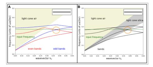
**Figure 5.6:** Illustration of guided modes in a slab waveguide. The dimensions of the waveguide are given in Table 4.1. The width of the waveguide is set to 500 nm. The substrate for the structure simulated in Figure **A** is simulated as air. The substrate for the structure simulated in Figure **B** is simulated as silica. The dispersion relation for both structures are is simulated along the waveguide length. Wavevector  $k_x$  is given in units of  $2\pi a/\lambda_x$ .
