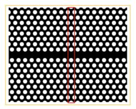
**Figure 4.3:** Illustration of the structure created when calculating the bands for a line defect in triangular PC. The red rectangle represent the simulation cell. The Master Equation is solved for wavevectors along the line defect. It is sufficient to compute for the wavevectors from  $\Gamma$  to K'.  $\Gamma$  is located in the center of the computational cell, K' at each end of the computational cell and within the line defect.
