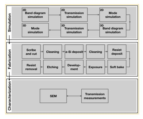
Figure 4.1: Schematic illustration for the experimental procedure of producing PCRRs.
