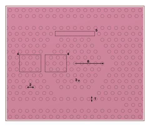
Figure 1.4: Overview of areas of interest for optimization. 1 refers to the separation distance between ring-resonator and waveguide. 2 refers to the lattice constant. 3 refers to the air-hole radius. 4 refers to the ring resonator corners. 5 refers to the ring resonator line defects. 6 refers to the ring resonator radius.
