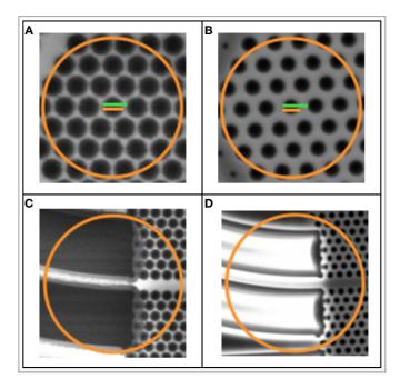
**Figure 5.18:** Four SEM-images of two different samples are illustrated. Figures **A** and **C** represent a sample etched for 77 seconds. Figures **B** and **D** represent a sample etched for 47 seconds. Yellow circles represent points of interest. The yellow and green lines captures hole diameter and lattice constant, respectively.
