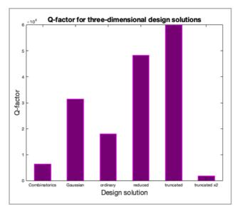
Figure 5.14: Diagram of Q-factors for all design solutions simulated in three-dimensions and with air as substrate.
