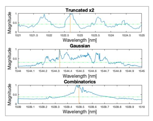
**Figure 5.23:** Transmission measurements focused in on most prominent frequency component for design solutions truncated x2, gaussian and combinatorics. The wavelength resolution varies from spectrum to spectrum.
