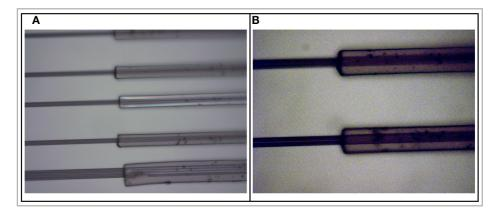
Figure 5.19: Images of inverted tapers captured with an optical microscope. Figures A and B represent the same inverted tapers. The magnification in Figures A and B are 20x and 100x, respectively.
