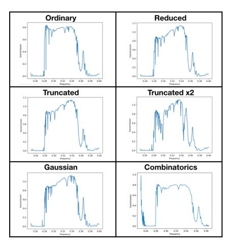
Figure 6.3: Transmission plots for three-dimensional design solutions. The frequency is normalized with respect to the lattice constant a and speed of light  $c (\omega a/2\pi c)$ .
