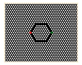
**Figure 4.6:** Simulation structure for resonant mode simulations. Red marker illustrates source position. Green marker illustrates the position of a harminv detector. A harminv detector detects the damping of a mode (i.e. the q-factor).
