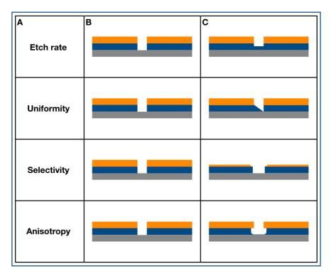
**Table 3.1:** Table illustrating the figures of merit. Yellow and blue colors are identical to Figures 3.5 and 3.7 illustrating resist and substrate, grey color illustrates part of substrate that is not intended to be etched. Column **A** is the figure of merit, column **B** illustrates the ideal etch case and is identical for each row, and column **C** illustrates a poor etch case due to the respective figure of merit.
