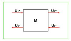
Figure 2.4: Illustration of a linear system represented by a M-matrix relating the output potential fields to the input potential fields. The potential field U is representing either an E- or H-field.
