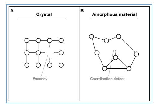
Figure 3.4: Illustration of defects in Silicon. Figure A illustrates c-Si and its simplest defect, vacancy. Figure B illustrates a-Si and its simplest defect, coordination defect.
