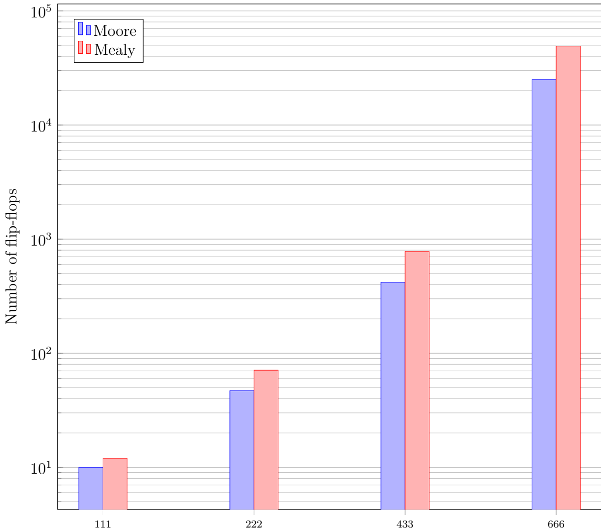
Figure 5.3: Number of flip-flops for different LUT sizes of LFSM. X-axis numbers are \{\#input\ width, \#state\ bits, \#output\ width\} , Y-axis is logarithmic with base 10.
