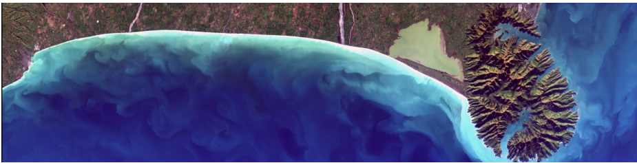
Figure 1.1: A three color-composite of three spectral bands taken from the hyperspectral dataset [2]. Image shows the coast of New Zealand recorded with Hyperspectral Imager for the Coastal Ocean (HICO) spectrometer.
