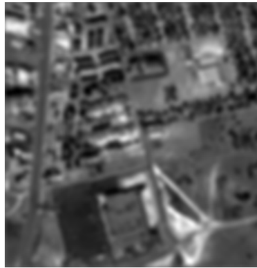
(b) Image degraded by the Gaussian PSF with \sigma = 2.3 .
