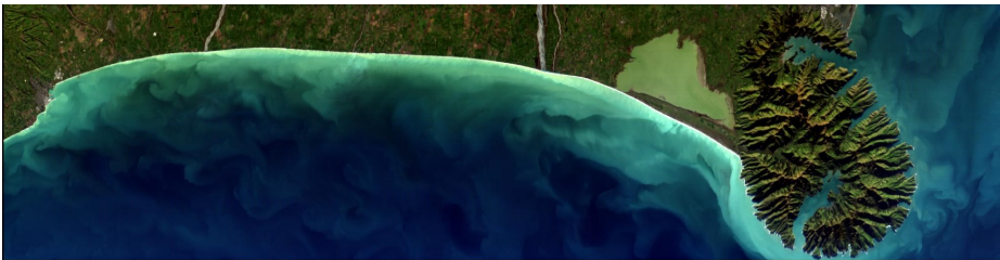
Figure 3.2: Image to the left shows a three-color composite of three spectral bands (18, 25, 53) from HICO data set [2].
